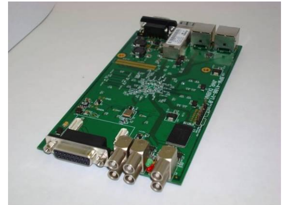
One of 30 chips (hi-tech) for automatic system for beam orbit measurement
