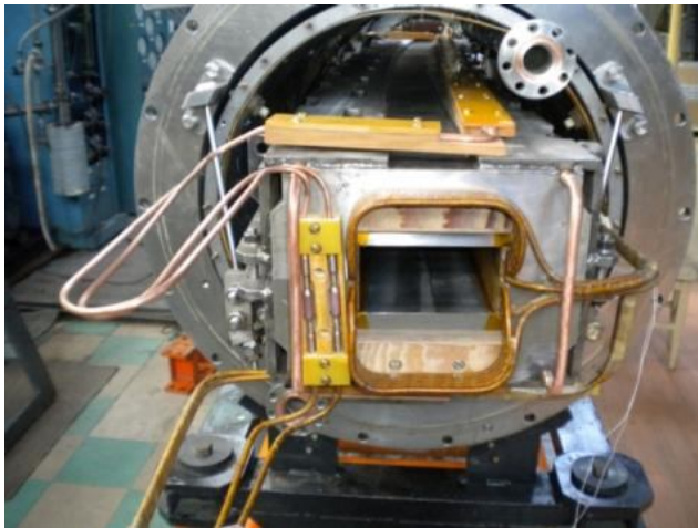
Installation of the cryostat with the magnet on the bench for the cryogenic test.
