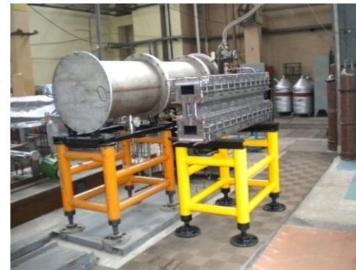
Collider dipole prototype magnet at vacuum tests
