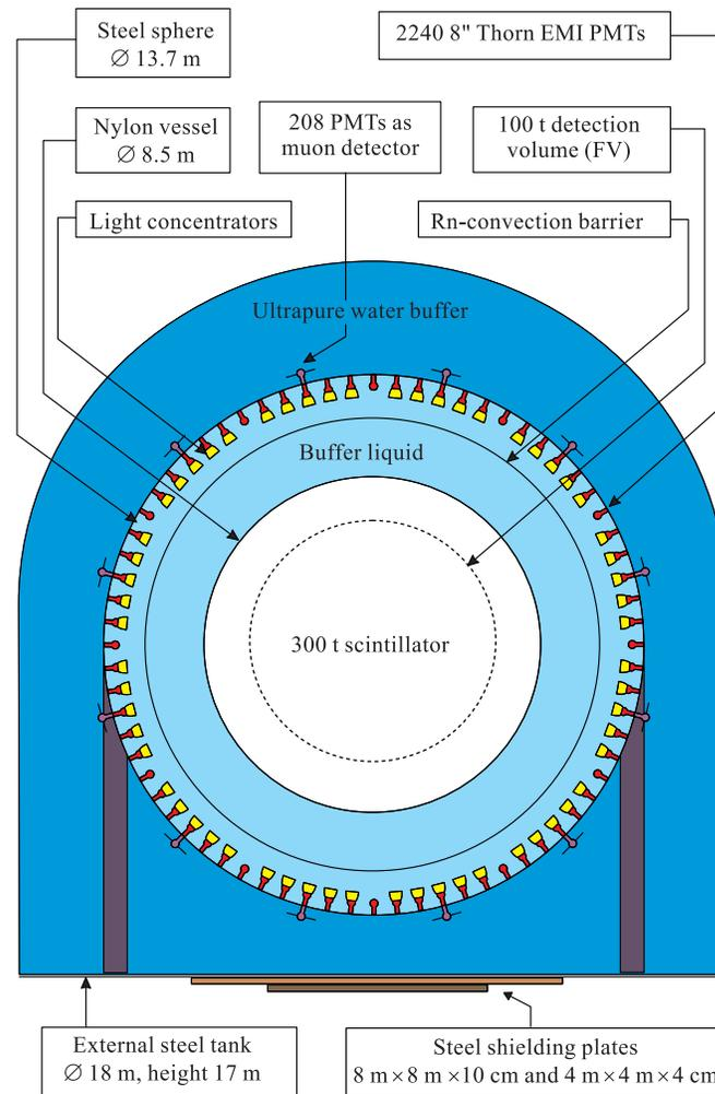
Fig. 2. Schematic view of the BOREXINO detector set-up, showing the most important structure elements of the detector
