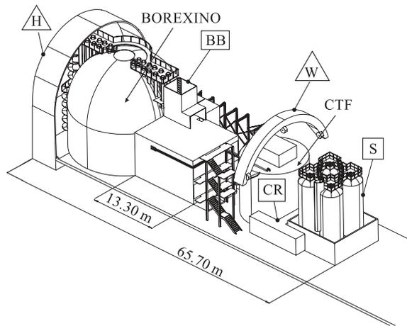
Fig. 1. Schematic overview of the Hall C at the Gran Sasso Underground Laboratory with the BOREXINO detector and the Counting Test Facility (CTF) [17]: H — tunnel walls of the Hall C; W — movable crane; CR — clean room of the CTF; S — storage vessel area for the liquid scintillator; BB — big building with electronic equipment, clean rooms, etc.
