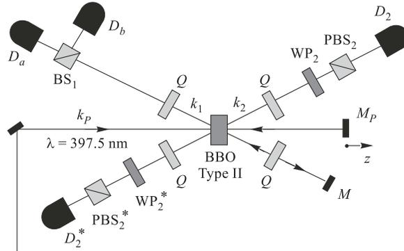
Fig. 4. Experimental realization of the quantum U-NOT gate
