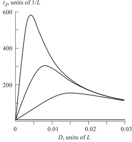
The Zeno time  $t_Z$  as the function of the energy difference  $\Delta$  for two-level Friedrichs model. The parameters of the model are:  $\Lambda = 8.498 \cdot 10^{18} \text{ s}^{-1}$ ,  $\omega = 1.55 \cdot 10^{16} \text{ s}^{-1}$ ,  $\lambda^2 = 6.43 \cdot 10^{-9}$ . From above, the curves correspond to the initial condition  $\Phi$ :  $(\alpha_1, \alpha_2) = (1, -0.6)$ ,  $(1, 1)$ ,  $(1, 0.1)$  and  $(1, 0)$ , respectively
