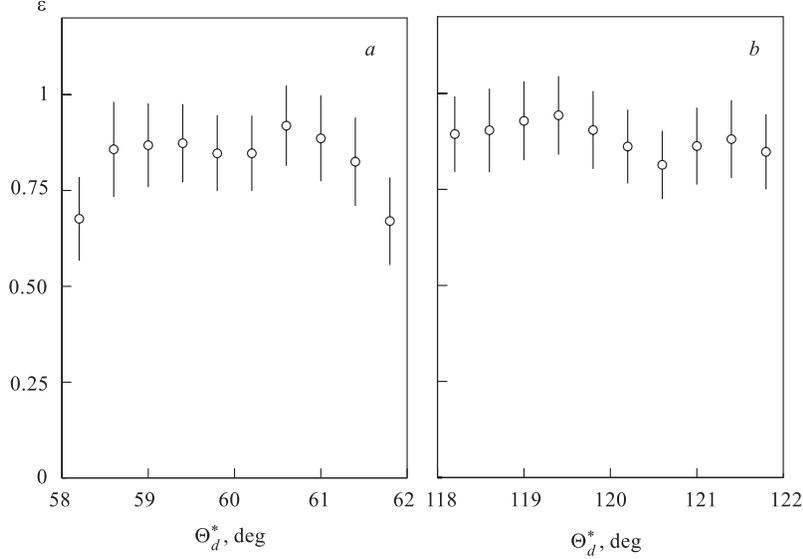
Fig. 3. Efficiency of the  $dp$  elastic-events detection versus deuteron scattering angle in c.m. in the case of lead degrader thickness for proton arm of 1.33 cm (a) and for deuteron arm of 1.56 cm (b)
