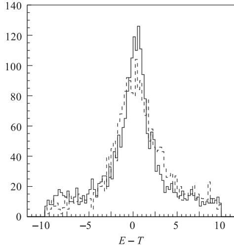
Fig. 8. The difference between the real and reconstructed energies of undetected neutron in the  $dp \rightarrow ppn$  reaction at 500 MeV and at  $\pm 40^\circ$  proton emission angles. The solid and dashed lines are obtained without and with 1.5 cm Pb degrader, respectively
