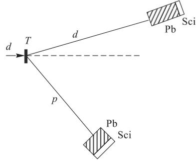
Fig. 2. Layout of the two-arm detector for the  $dp$  elastic-scattering experiment: T is the target; Sci are the scintillators; Pb are the lead degraders
