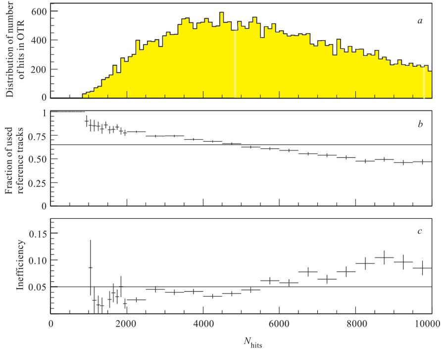
Fig. 7. Dependence of the PC chambers track-finding inefficiency on the number of hits
