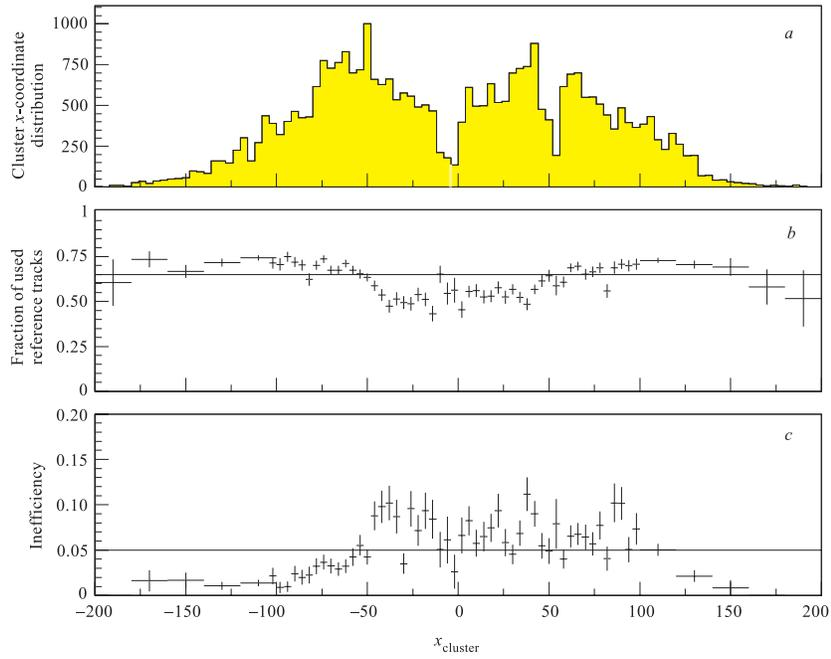
Fig. 9. Dependence of the PC chambers track-finding inefficiency on the  $x$  coordinate of ECAL cluster
