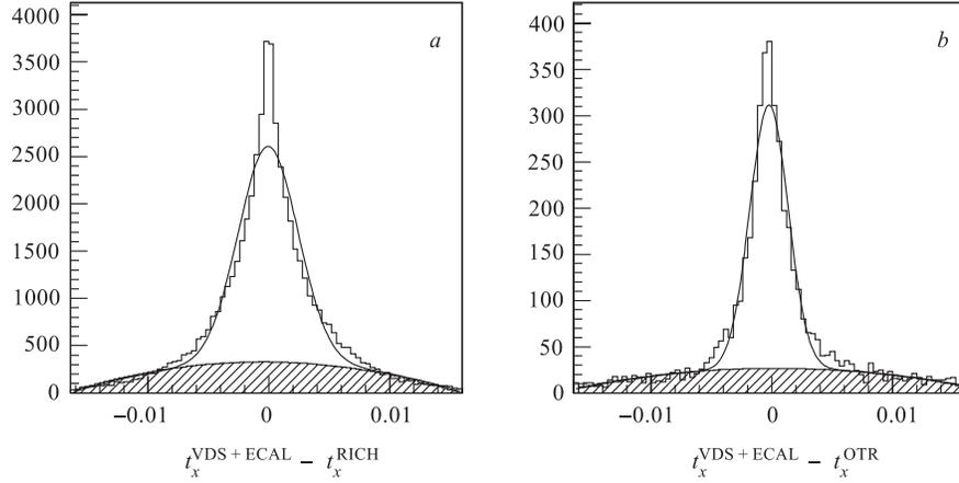
Fig. 3. Distributions of the slope differences used to estimate the ghost rates for the VDS+RICH+ECAL track reconstruction (a) and for matching PC segment with the VDS+RICH+ECAL track (b). The dashed area is considered as the ghost contribution
