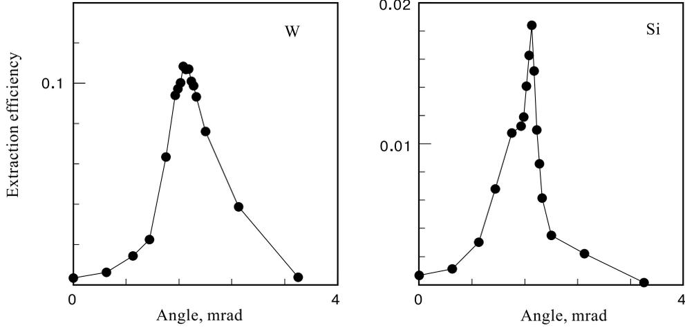
Fig. 4. The dependence of the extraction efficiency of circulating deuterons from the Nuclotron on the orientation angle of the silicon and tungsten crystals. The crystal bending radius, length and thickness are 10cm, 1 cm and 100  $\mu\text{m}$ , respectively
