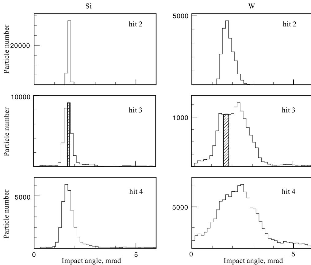
Fig. 2. The distributions in impact angles of deuterons with the crystals. The conditions are the same as for Fig. 1. The dashed parts of the histograms show the angular regions where particles can be captured into channeling states
