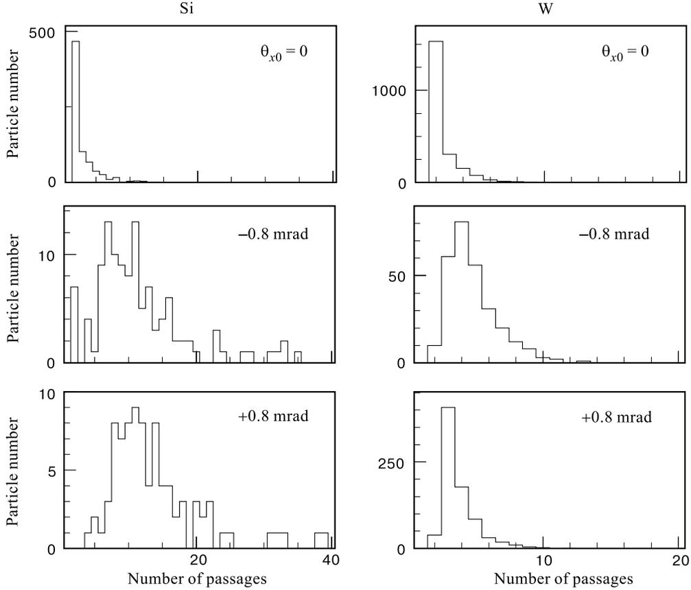
Fig. 3. The distributions of extracted particles in the number of passages through the crystal for different angles of the crystal relative to the beam envelope slope
