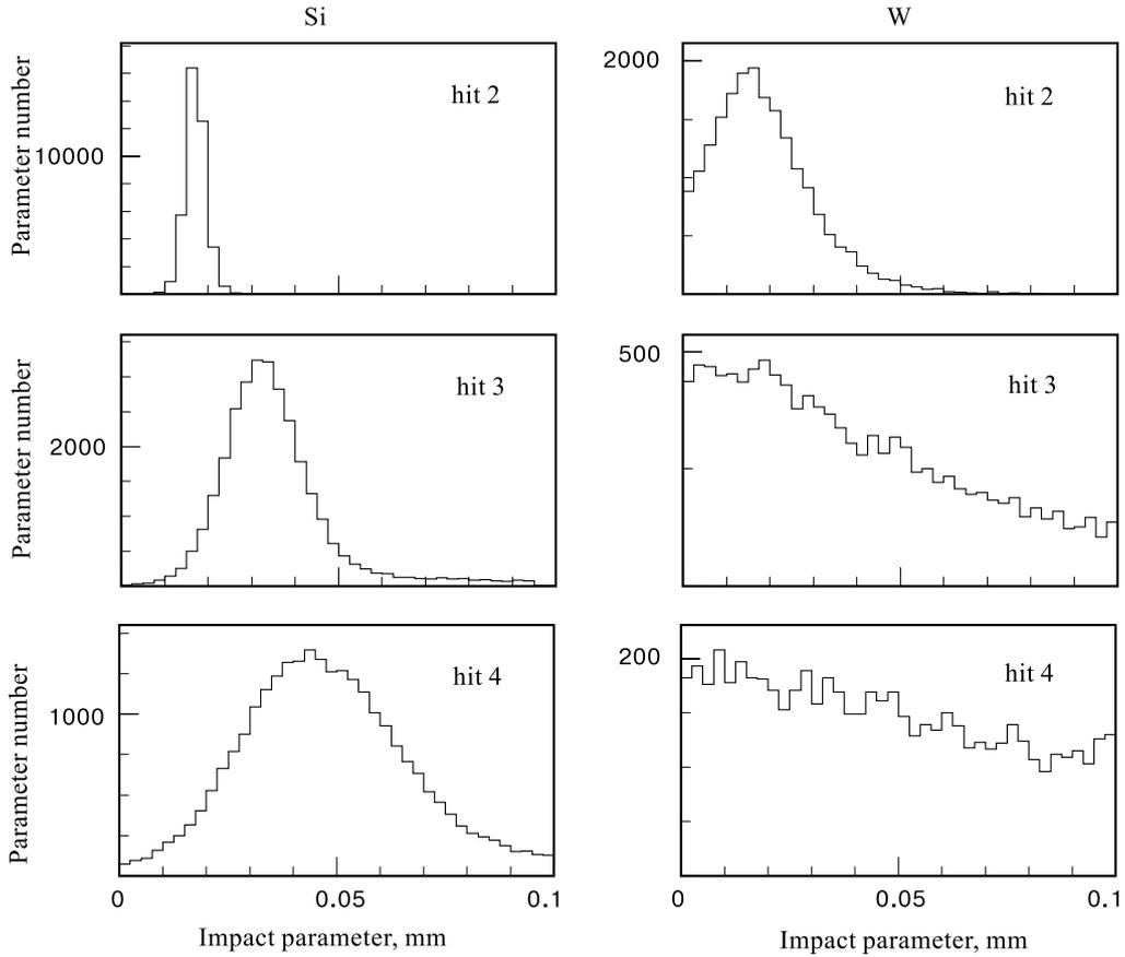
Fig. 1. The distributions in impact parameters of deuterons with the energy of 6 GeV/u of the Nuclotron circulating beam for the second, third and fourth hits in the silicon and tungsten crystals
