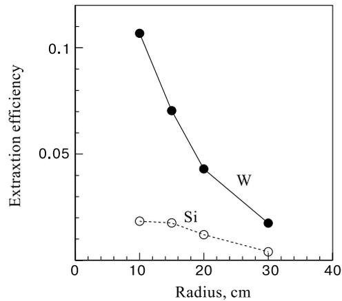
Fig. 8. The extraction efficiency as a function of the bending radius of the crystal. The crystal thickness is  $100 \mu\text{m}$
