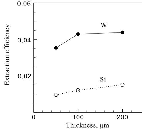
Fig. 5. The dependence of the extraction efficiency of deuterons from the Nuclotron on the crystal thickness. The crystal bending radius and length are 20cm and 2 cm
