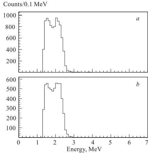
Fig. 1. Energy spectra of two-electron events for enriched (651.4 kg·h) (a) and natural (441.1 kg·h) molybdenum (b)
