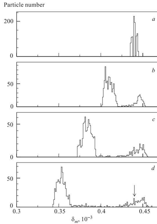
Fig. 12. The distributions of halo particles in amplitudes  $\delta_m$  under the action of the resonance damping sequence at different turn numbers:  $50 \cdot 10^3$  (a),  $250 \cdot 10^3$  (b),  $450 \cdot 10^3$  (c),  $750 \cdot 10^3$  (d). The pulse duration  $\Delta l_p = 2$  cm,  $V_p = 0.5$  MV,  $N_{on} = 640$ . The arrow shows the initial amplitude of particles
