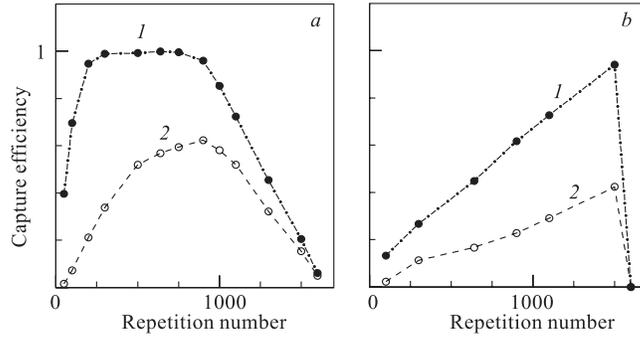
Fig. 6. The dependence of the capture efficiency (1) of halo particles by the resonance strengthening sequence and their ejection efficiency from the bucket (2) on the repetition number with using accelerating (a) or decelerating (b) pulses. The initial amplitude  $\delta_{m0} = 0.35 \cdot 10^{-3}$ , the pulse duration  $\Delta l_p = 2$  cm
