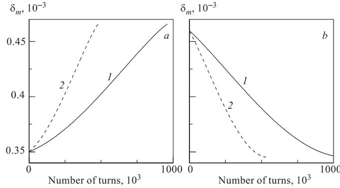
Fig. 2. The oscillation amplitude  $\delta_m$  as a function of turn number for a halo particle driven by a single resonance sequence. *a*) For the strengthening sequence,  $\delta_{mo} = 0.35 \cdot 10^{-3}$ . *b*) For the damping sequence,  $\delta_{mo} = 0.46 \cdot 10^{-3}$ . The curves 1 and 2 are for the pulse voltage  $V_p = 0.5$  MV and 1 MV correspondingly
