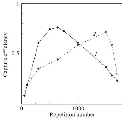
Fig. 13. The dependence of the capture efficiency of halo particles by the damping sequence on the repetition number. The initial amplitude  $\delta_{m0} = \delta_{ms}$ , where  $\delta_{ms} = 0.44 \cdot 10^{-3}$  is the start amplitude of the sequence. The pulse length  $\Delta l_p = 2$  cm,  $V_p = 0.5$  MV. The curve 1 and 2 are for decelerating and accelerating pulses correspondingly
