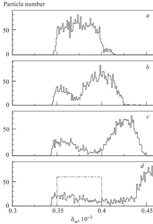
Fig. 7. The distributions of halo particles in amplitudes  $\delta_m$  under the action of the resonance strengthening sequence at different turn numbers:  $25 \cdot 10^3$  (a),  $225 \cdot 10^3$  (b),  $325 \cdot 10^3$  (c),  $425 \cdot 10^3$  (d). The initial distribution with  $\delta_{m0} = (0.35-0.40) \cdot 10^{-3}$  is uniform (dashed line). The pulse length  $\Delta l_p = 5$  cm,  $N_{on} = 1500$
