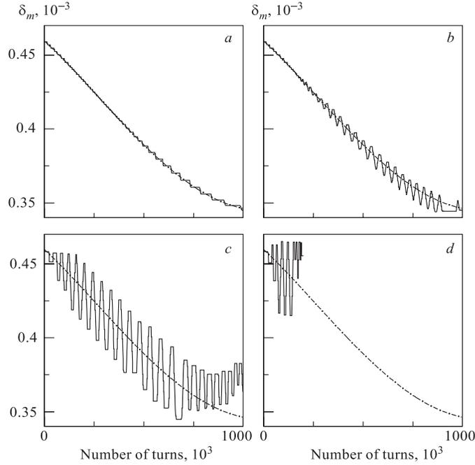
Fig. 11. The oscillation amplitude  $\delta_m$  as a function of turn number for a halo particle driven by a resonance damping sequence with different pulse length  $\Delta l_p$  and repetition number  $N_{on}$ . With short pulses  $\Delta l_p = 2$  cm,  $N_{on} = 100$  (a), 1500 (b). With long pulses  $\Delta l_p = 10$  cm (c) and 20 cm (d),  $N_{on} = 640$ . The pulse voltage  $V_p = 0.5$  MV
