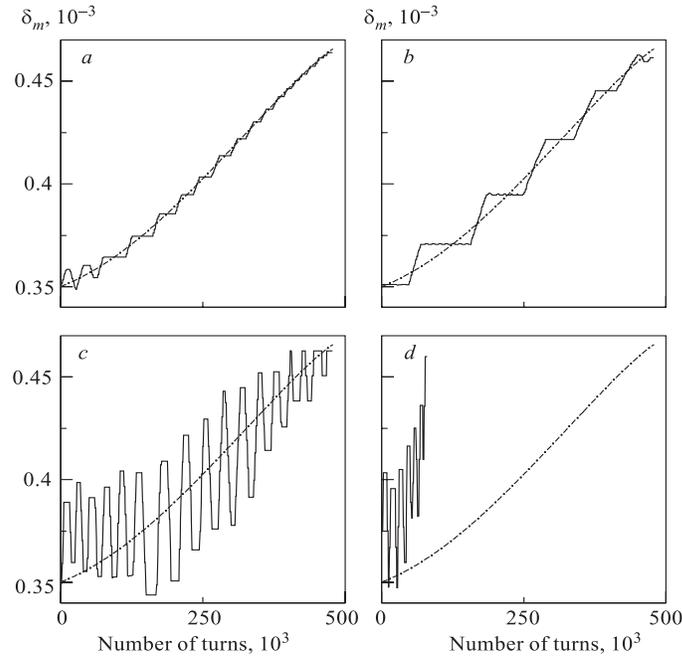
Fig. 4. The oscillation amplitude  $\delta_m$  as a function of turn number for a halo particle driven by a resonance strengthening sequence with different pulse length  $\Delta l_p$  and repetition number  $N_{on}$ . With short pulses  $\Delta l_p = 1$  cm,  $N_{on} = 100$  (*a*), 1500 (*b*). With long pulses  $\Delta l_p = 10$  cm (*c*) and 20 cm (*d*),  $N_{on} = 640$ . The pulse voltage  $V_p = 1$  MV. The dash-dotted line is for a single resonance sequence
