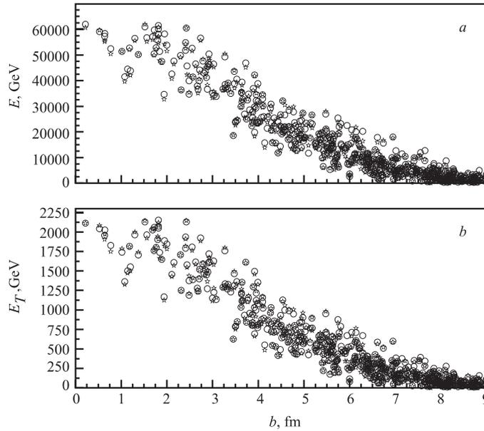
Fig. 12. Correlation between the total (a) and transverse (b) energy deposition in HF and impact parameter of 500 minimum bias Ar–Ar collisions: HIJING predictions (stars) and reconstructed responses (open circles)
