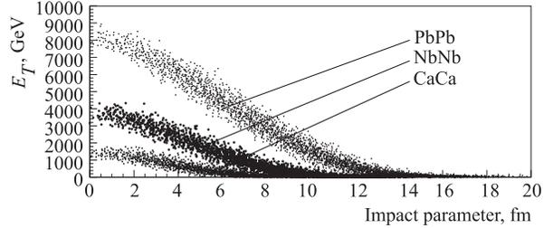
Fig. 2. Correlation between the transverse energy flow  $E_T$  in the very forward rapidity  $3 \leq |\eta| \leq 5$  and collision impact parameter  $b$ . From top to bottom: Pb–Pb, Nb–Nb, Ca–Ca collisions at  $\sqrt{s} = 5.5A$  TeV
