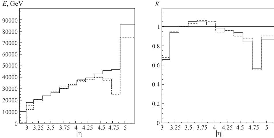
Fig. 10. HIJING total energy  $E(\text{hijing})$  in central Pb–Pb collisions (solid histogram) and HF calorimeter response  $E(l + s)$  (the sum of energies in towers with long and short fibers) for the cases with (dashed histogram) and without (dash-dotted histogram) CMS magnetic field  $B = 4$  T
