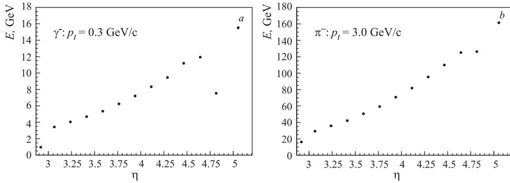
Fig. 8. The reconstructed energy deposition in the ring as the function of  $\eta$  for  $\gamma$  photons with  $p_t = 0.3 \text{ GeV/c}$  (a) and  $\pi^-$  with  $p_t = 3.0 \text{ GeV/c}$  (b)
