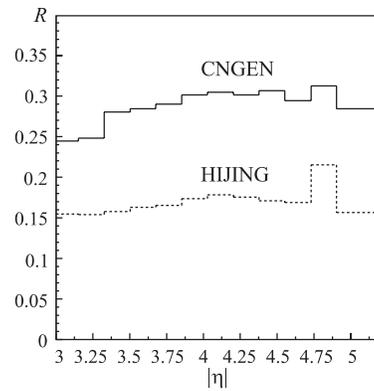
Fig. 15. The «short fiber»-to-«long fiber» energy deposition ratio  $R$  in HF towers for Centauro (solid histogram) and HIJING (dashed histogram) central Pb–Pb events
