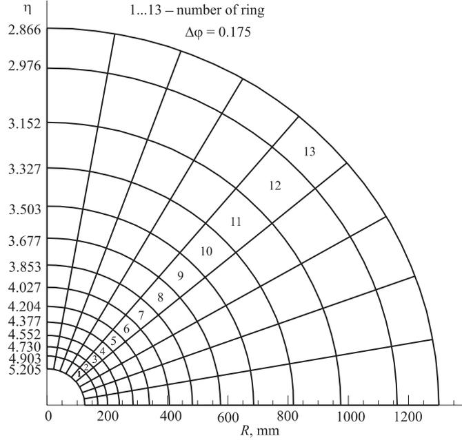
Fig. 7. Hadron Forward Calorimeter: the transverse view
