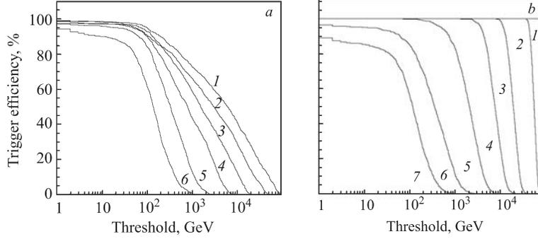
Fig. 6. The efficiency of the event selection: *a*) for minimum bias nucleus-nucleus collisions: 1 — PbPb; 2 — NbNb; 3 — CaCa; 4 — OO; 5 —  $\alpha\alpha$ ; 6 —  $pp$ ; *b*) for Pb–Pb collisions at various impact parameter intervals (fm): 1 — 0...2; 2 — 4...6; 3 — 8...10; 4 — 10...12; 5 — 12...14; 6 — 14...16; 7 — 16...18
