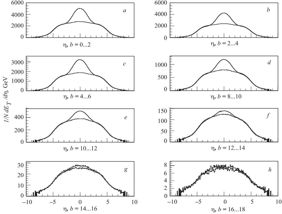
Fig. 1. Normalized differential distribution of the total transverse energy  $dE_T/d\eta$  over pseudorapidity  $\eta$  for 10,000 minimum bias Pb–Pb collisions at  $\sqrt{s} = 5.5A$  TeV for various impact parameters. The two cases are included: with jet quenching (the top line) and without jet quenching (the lower line)
