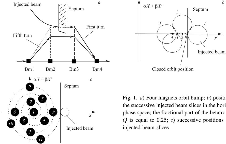
Fig. 1. *a)* Four magnets orbit bump; *b)* positions of the successive injected beam slices in the horizontal phase space; the fractional part of the betatron tune  $Q$  is equal to 0.25; *c)* successive positions of the injected beam slices
