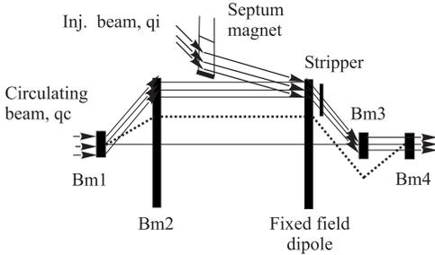
Fig. 4. Stripping injection of heavy ions into Nuclotron booster
