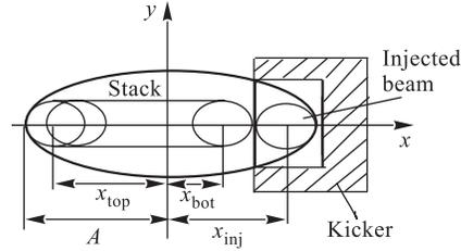
Fig. 3. Principle of RF stacking
