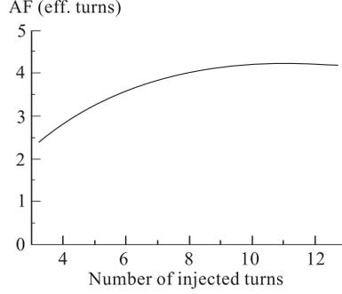
Fig. 2. Accumulation factor for multi-turn injection versus the number of injected turns
