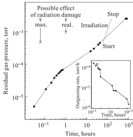
Fig. 5. Residual gas pressure inside the vacuum container as a function of time. The figure inserted shows the outgassing rate behaviour over the same period of time
