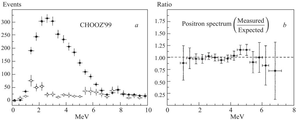
Fig. 2. CHOOZ positron energy spectrum: *a*) spectra in reactor ON and OFF periods; *b*) measured to expected no-oscillation ratio
