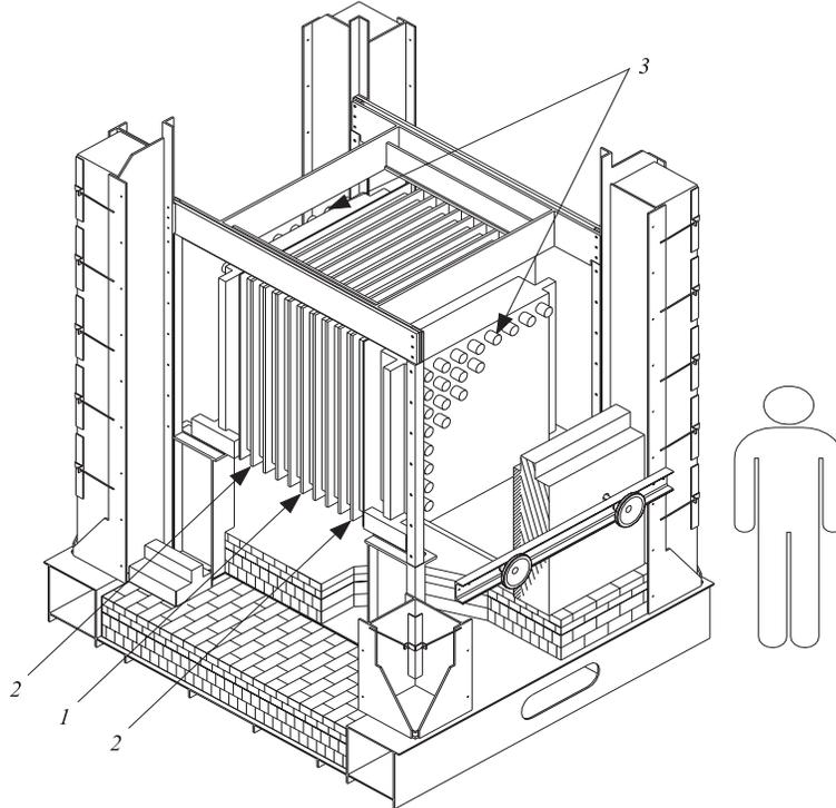
Fig. 2. The NEMO-2 detector without shielding: 1 — central frame with the source plane capable of supporting plural source foils; 2 — ten frames of 2 × 32 Geiger cells for tracking; 3 — scintillator array
