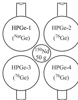
Fig. 1. Top view of the HPGe detector assembly with the  $^{150}\text{Nd}$  sample
