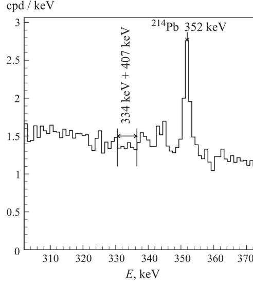
Fig. 5. A fragment of the experimental one-dimensional spectrum near the  $^{150}\text{Nd}(2\beta, 2\nu + 0\nu)^{150}\text{Sm}(0_1^+)$  region of interest
