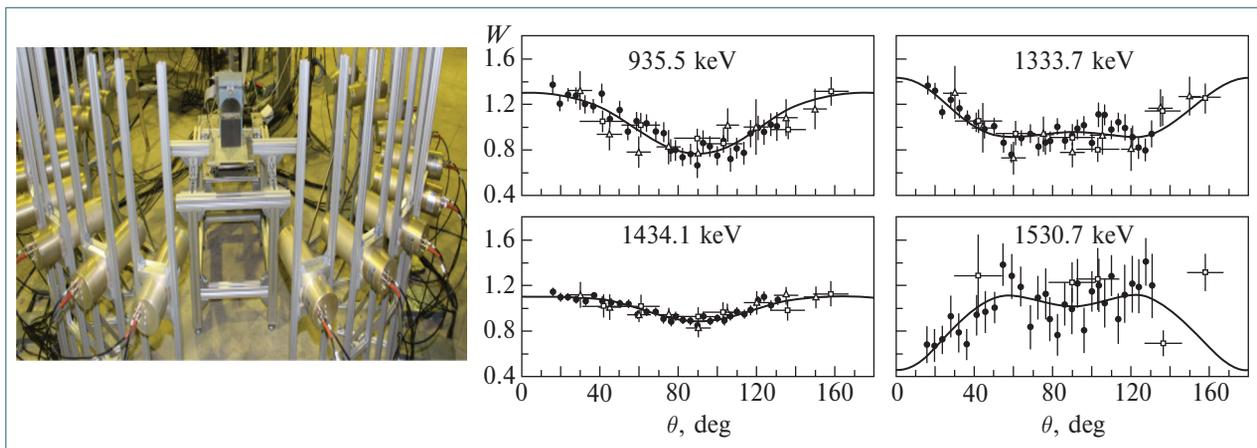
Left: TANGRA facility with 18 BGO scintillation detectors. Right: angular distributions of  $\gamma$  rays for transitions in  $^{52}\text{Cr}$ . Solid curves are data approximation by Legendre polynomials
