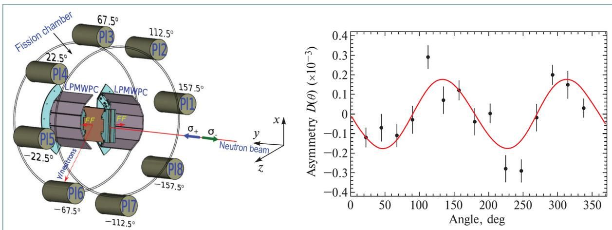
Left: scheme of the experimental facility. Right: asymmetry coefficient for  $\gamma$  rays as a function of the emission angle relative to the fission axis in the resonance of  $^{235}\text{U}$  (0.3 eV)
