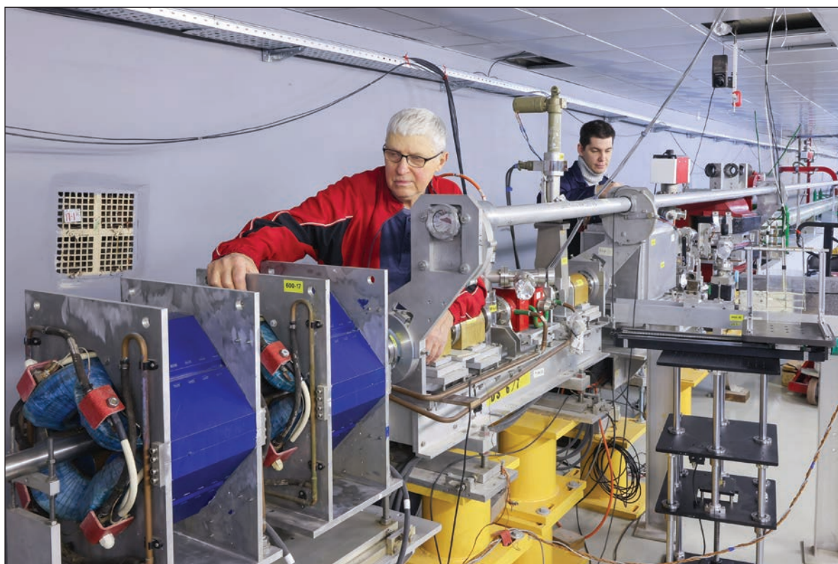
The Dzhelepov Laboratory of Nuclear Problems. Adjustment of the vacuum system of the LINAC-200 electron accelerator
