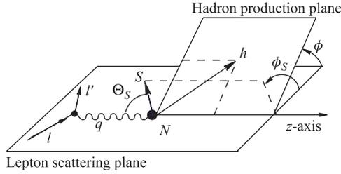
Fig. 1. Kinematics of the process  $lN^{\uparrow} \rightarrow l'hX$  in the lab. frame
