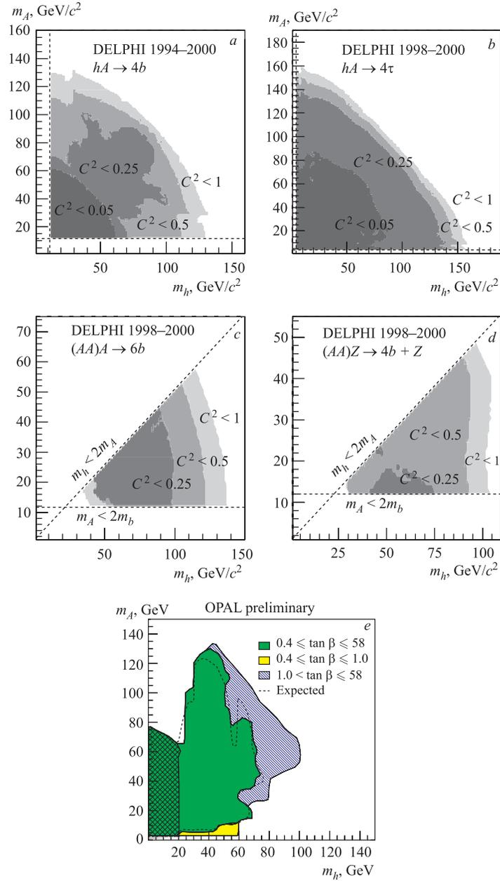
Fig. 22. 2DHM. *a, c*) Mass limits from dedicated searches for  $hA$  production.  $C^2$  is the reduction factor on the maximum production cross section. *b, d*) Mass limits from a general 2DHM parameter scan
