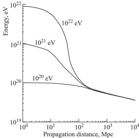
Fig. 2. Dependence of energy of a proton as a function of distance traveled, for different initial energies [8]
