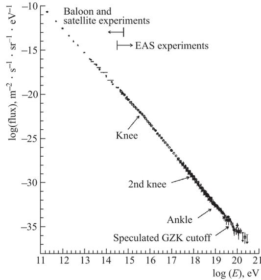
Fig. 1. Energy spectrum of cosmic rays compiled from results of various experiments. The energy ranges of direct measurements (on balloons and satellites) and indirect ones (extensive air shower detection) are shown [2]
