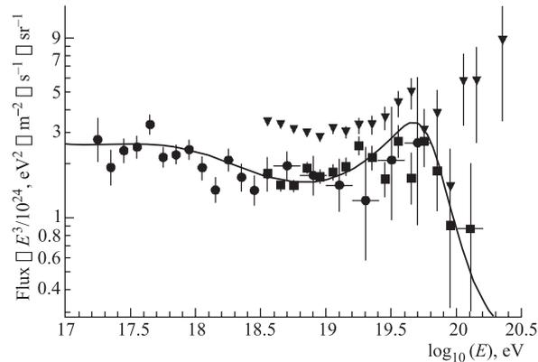
Fig. 4. Cosmic ray energy spectra determined in the AGASA and HiRes experiments [36]. The line shows predictions of the model [38] fitted to the HiRes spectrum. ● — HiRes-2 monocular; ■ — HiRes-1 monocular; ▼ — AGASA
