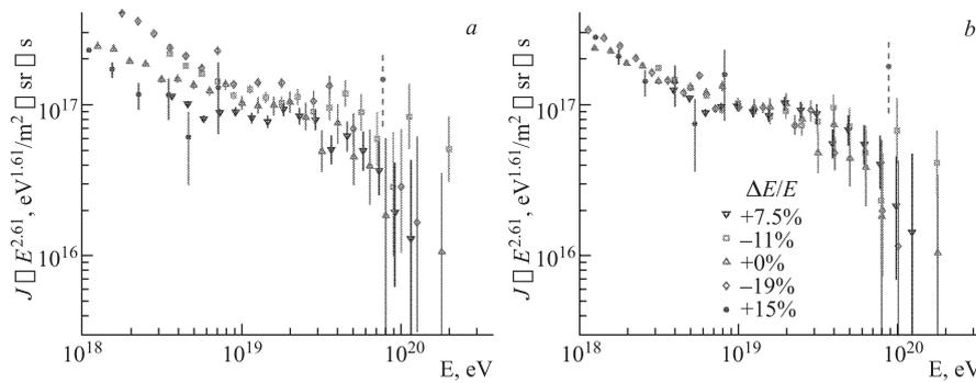
Fig. 6. Comparison of energy spectra from different experiments [40]. *a*) The spectra as published by AGASA (□), Fly's Eye (△), Haverah Park (●), HiRes (▽) and Yakutsk (◇). *b*) The same spectra after rescaling the energy calibration in the experiments to bring the spectra into agreement at 10 EeV
