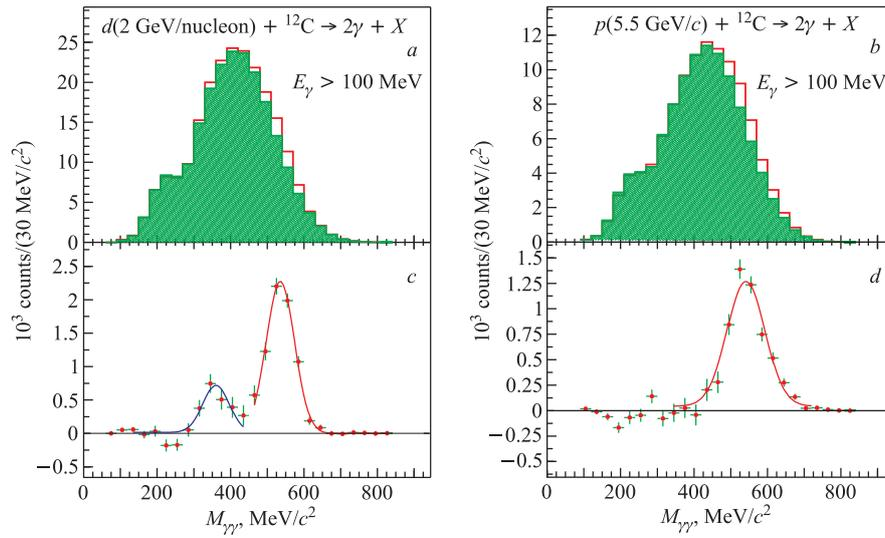
Fig. 2. Invariant mass distributions of  $\gamma\gamma$  pairs satisfying criteria 1)–3) and the trigger condition without (*a, b*) and with (*c, d*) the background subtraction. The plots *a, c* and *b, d* are obtained for the reaction *dC* collision at 2.75 GeV/*c* per nucleon and *pC* collision at 5.5 GeV/*c*, respectively. The curves are the Gaussian approximation of experimental points
