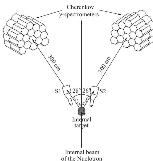
Fig. 1. The schematic drawing of the experimental PHOTON-2 setup. The S1 and S2 are scintillation counters
