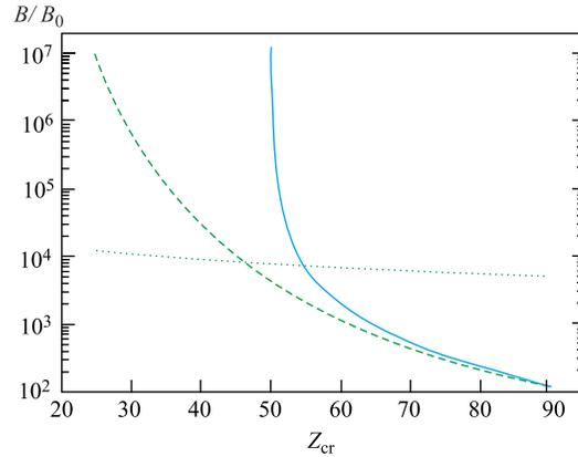
Fig. 2. The values of  $B_{cr}^Z$ : without screening according to [7], dashed line; numerical results with screening, solid line. The dotted line corresponds to the field at which  $a_H$  becomes smaller than the size of the nucleus
