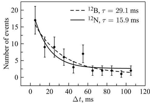
Fig. 5. Exponential decay curves  $\sim e^{-t/\tau}$  for  ${}^{12}\text{B} \rightarrow {}^{12}\text{C} + e^- + \bar{\nu}_e$  (dashed) and  ${}^{12}\text{N} \rightarrow {}^{12}\text{C} + e^+ + \nu_e$  (solid). The solid circles are the experimental data of the BUST taken in 2012
