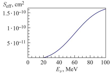
Fig. 4. Effective area of the BUST for the reaction  $\nu_e + {}^{12}\text{C} \rightarrow {}^{12}\text{N} + e^-$
