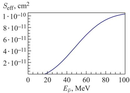
Fig. 3. Effective area of the BUST for the reaction  $\bar{\nu}_e + {}^{12}\text{C} \rightarrow {}^{12}\text{B} + e^+$
