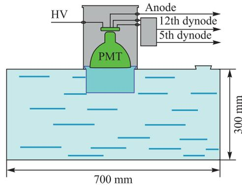
Fig. 2. A standard scintillation detector of the BUST
