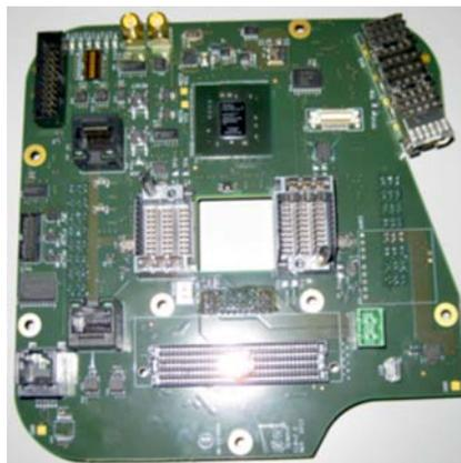
Fig. 8. Picture of the DOM Central Logic Board
