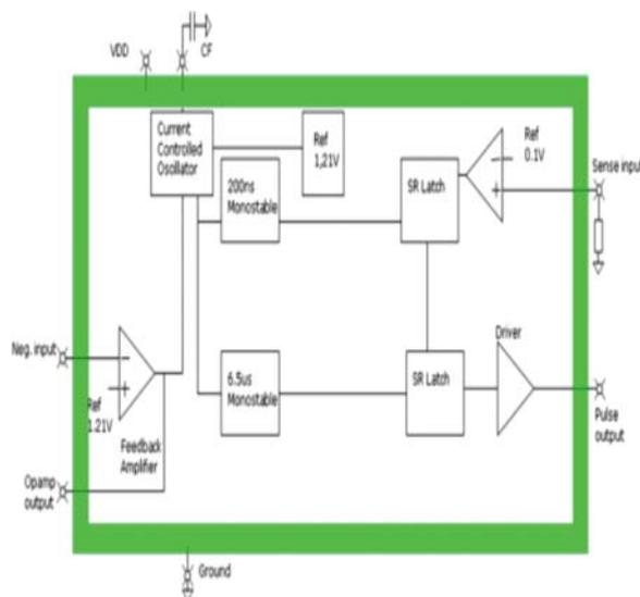
Fig. 5. Block diagram of the CoCo chip
