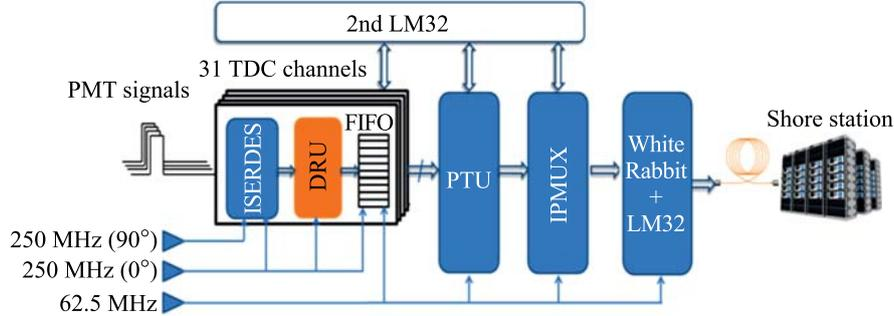
Fig. 11. Complete readout architecture
