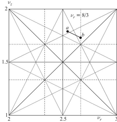
Fig. 8. The USR betatron tune diagram. Shown are: *a* — operation point of circulating beam  $\nu_r = 2.5443$  and  $\nu_z = 1.7905$ ; *b* — excited resonance  $\nu_r = 2.6637$  and  $\nu_z = 1.7315$  in the process of slow extraction. Also shown are I, II, III, IV operation points of original USR design [2]
