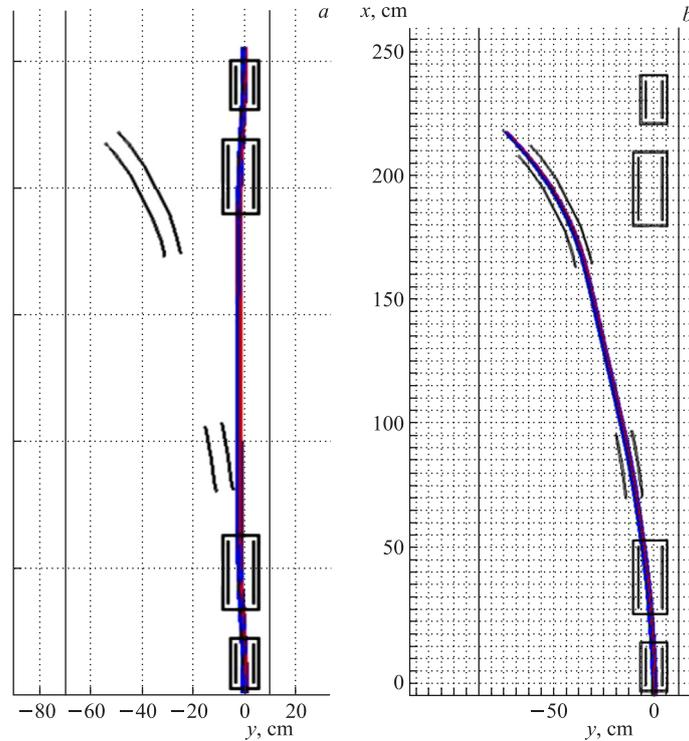
Fig. 6. Ion trajectories in the extraction section: *a*) circulating beam in the bump region; *b*) extracted beam
