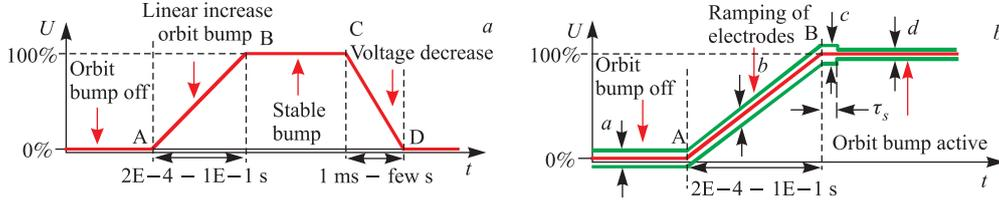
Fig. 7. Chronological sequence of orbit bump operation: *a*) A, B, C, D are the points where voltage starts to rise up or fall down; *b*) voltage offset during ramping, shown are «*a*» and «*d*» voltage stability at plateau  $\Delta U/U = \pm 1 \cdot 10^{-4}$ , «*b*» and «*c*» voltage stability during transition and stabilizing period  $\Delta U/U = \pm 2 \cdot 10^{-4}$ , stabilizing time  $\tau_s < 100 \mu s$
