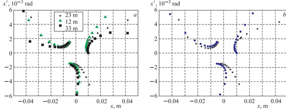
Fig. 10. Resonance extraction separatrices at the position of the electrostatic septum: *a*) different sextupole location at 12 m (triangles), at 23 m (stars) and at 33 m (squares); *b*) adjusting of separatrix arm orientation by simultaneous powering of two sextupoles  $k_{Sx} = -6 \text{ m}^{-2}$  at 12 m and  $k_{Sx} = +1 \text{ m}^{-2}$  at 23 m (stars) as well as  $k_{Sx} = +1 \text{ m}^{-2}$  at 12 m and  $k_{Sx} = -6 \text{ m}^{-2}$  at 23 m (circles)
