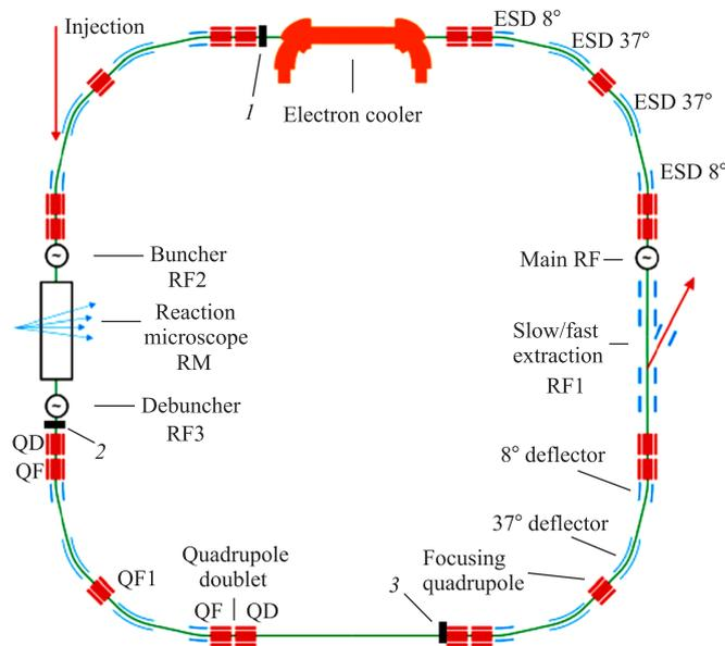
Fig. 1. Modified layout of the USR. Extraction section is outlined. Possible locations of sextupole for slow extraction: 1 — at 12 m; 2 — at 23 m; 3 — at 33 m
