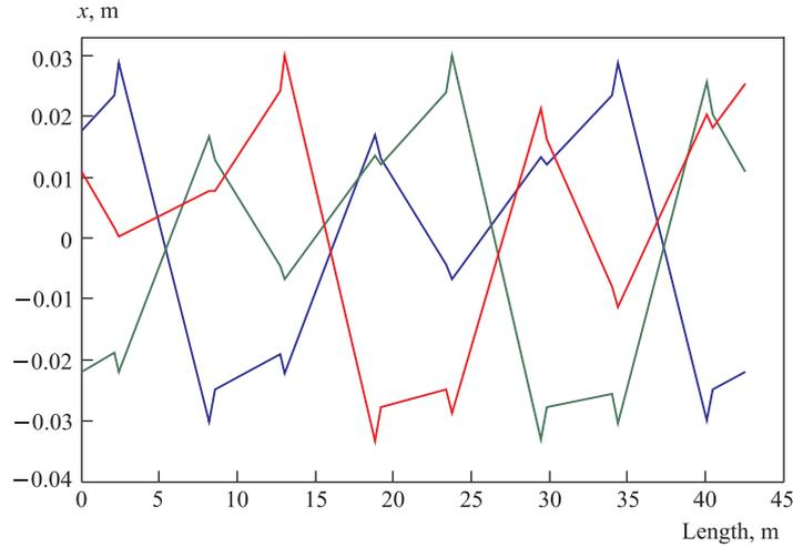
Fig. 11. The last three turns of the central particle in the ring during slow extraction
