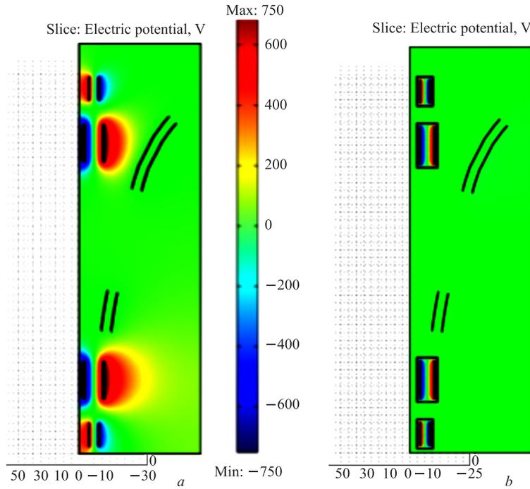
Fig. 4. Electric potential distribution in the model: *a*) original version without shields; *b*) modified model with shielded electrodes
