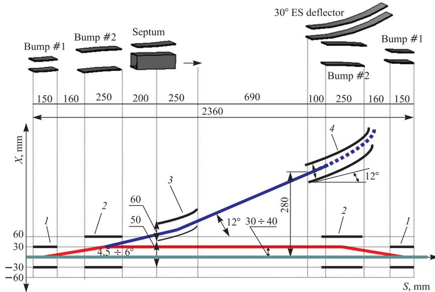
Fig. 2. Location of elements of the combined extraction systems in one of the USSR straight sections: 1 — parallel plate bump electrodes #1; 2 — parallel plate bump electrodes #2; 3 —  $6^\circ$  electrostatic septum deflector of cylindrical shape, entrance tilt angle to the axis is variable from 0 to  $6^\circ$ ; 4 —  $30^\circ$  electrostatic deflector
