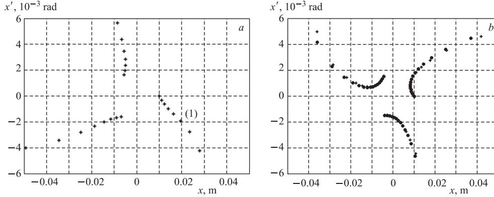
Fig. 9. Slow extraction phase space diagrams at the position of the electrostatic septum. The sextupole is located at 23 m: *a*) sextupole strength is  $k_{Sx} = +5 \text{ m}^{-2}$  and outbound arm #1 has negative momentum, i.e., directed inward; *b*) sextupole strengths are  $k_{Sx} = -4 \text{ m}^{-2}$  (circles) and  $k_{Sx} = -5 \text{ m}^{-2}$  (stars). Outbound arms are directed outwards with positive momentum
