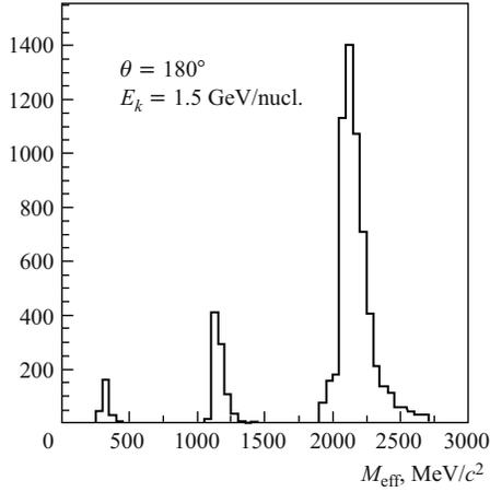
Fig. 3. Effective mass for coincidence of P and K arms
