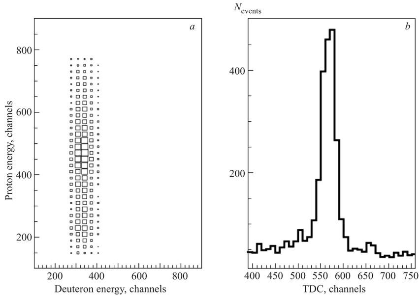
Fig. 3. The selection of the  $dp$ -elastic scattering events by the energy losses correlation (a) and time difference (b) after applying of the energy losses correlation criteria
