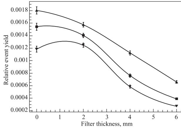
Fig. 8. Relative yield of selected  $dp$  events as a function of the filter thickness: ▲ — criteria A; ■ — criteria A + B; ▼ — criteria A + B with the background subtraction (curves are presented for better visualization)
