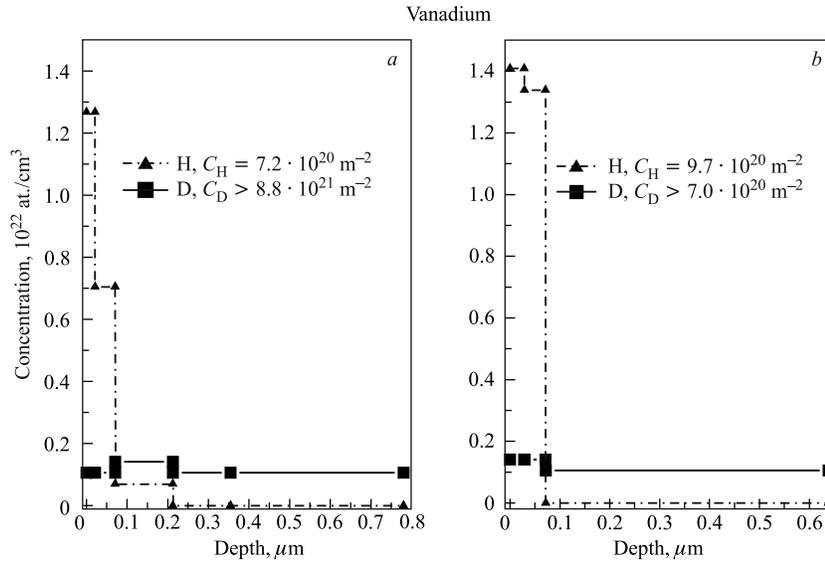
Fig. 6. The depth concentrations of D and H atoms in V samples after 25-keV  $D^+$  implantation at two fluences:  $\Phi_2 = 1.5 \cdot 10^{22} \text{ m}^{-2}$  (a) and  $\Phi_{\max} = 2.3 \cdot 10^{22} \text{ m}^{-2}$  (b). The  $D^+$  projected range is  $R_p = (1955 \pm 571) \text{ \AA}$
