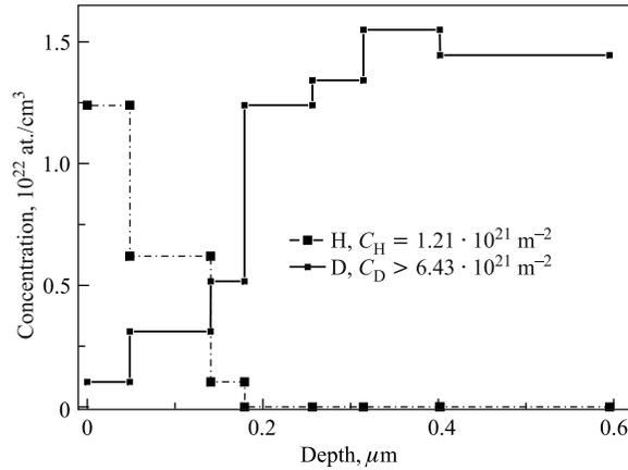
Fig. 4. The depth profiles of D and H atoms in  $\text{Al}_2\text{O}_3$  single crystal after 25-keV  $\text{D}^+$  implantation at fluence  $\Phi_{\text{max}} = 2.3 \cdot 10^{22} \text{ m}^{-2}$ . The  $\text{D}^+$  projected range is  $R_p = (2832 \pm 602) \text{ \AA}$
