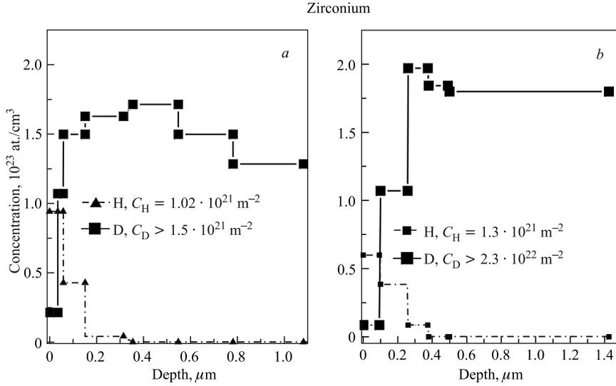
Fig. 2. The depth profiles of D and H atoms in Zr samples after 25-keV  $\text{D}^+$  implantation at two fluences:  $\Phi_2 = 1.5 \cdot 10^{22} \text{ m}^{-2}$  (a) and  $\Phi_{\max} = 2.3 \cdot 10^{22} \text{ m}^{-2}$  (b). Concentrations of the isotopes are given. The  $\text{D}^+$  ion projected range is  $R_p = (1923 \pm 643) \text{ \AA}$
