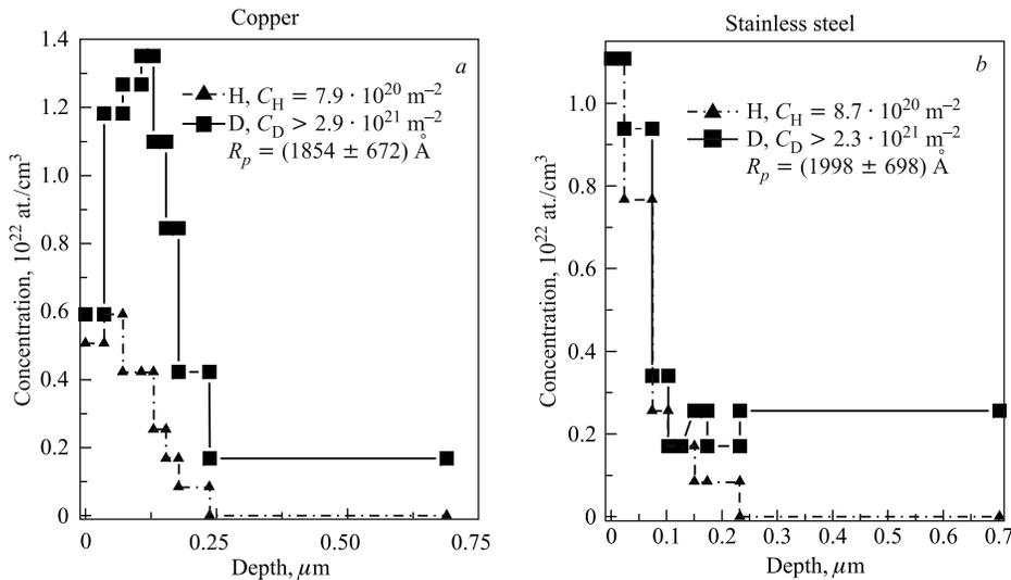
Fig. 5. The depth profiles of D and H atoms after 25-keV  $\text{D}^+$  implantation at one fluence  $\Phi_2 = 1.5 \cdot 10^{22} \text{ m}^{-2}$  in Cu (a) and stainless steel  $\text{Fe}_{72}\text{Cr}_{18}\text{Ni}_{10}$  (b) samples
