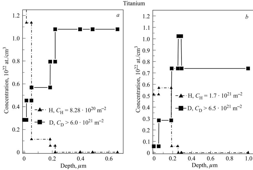
Fig. 3. The depth profiles of D and H atoms in Ti samples after 25-keV  $\text{D}^+$  implantation at two fluences:  $\Phi_2 = 1.8 \cdot 10^{22} \text{ m}^{-2}$  (a) and  $\Phi_{\text{max}} = 2.3 \cdot 10^{22} \text{ m}^{-2}$  (b). The  $\text{D}^+$  projected range is  $R_p = (2446 \pm 493) \text{ \AA}$
