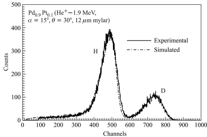
Fig. 1. The experimental ERDA and simulated spectra of H and D recoils in  $\text{Pd}_{0.9}\text{Pt}_{0.1}$  alloy implanted by 25-keV deuterium ions up to fluence  $\Phi_1 = 1.2 \cdot 10^{22} \text{ m}^{-2}$
