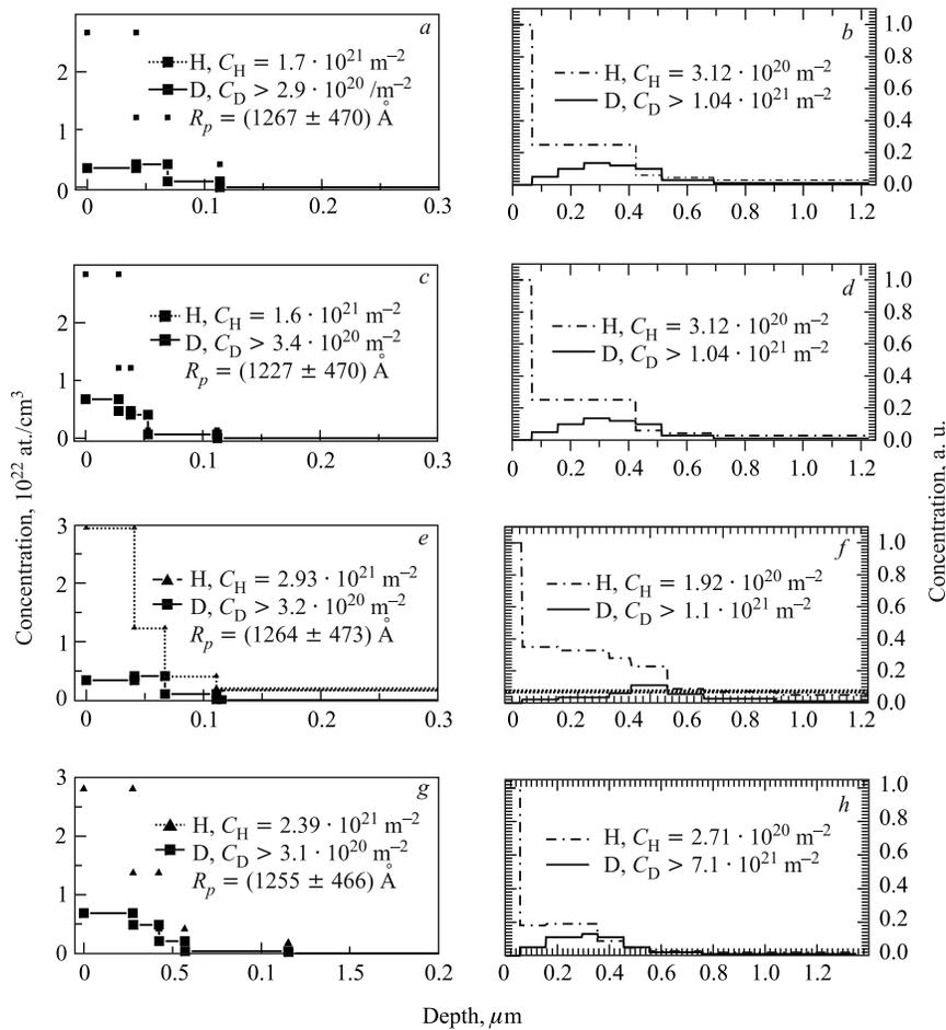
Fig. 8. The depth profiles of D and H atoms after 25-keV D<sup>+</sup> implantation at fluence  $\Phi_1 = 1.2 \cdot 10^{22} \text{ m}^{-2}$  in the following samples: Pd<sub>0.9</sub>Ag<sub>0.1</sub> (a, b); Pd<sub>0.9</sub>Pt<sub>0.1</sub> (c, d); Pd<sub>0.9</sub>Rh<sub>0.1</sub> (e, f); Pd<sub>0.9</sub>Ru<sub>0.1</sub> (g, h). The left column — 10 days; the right column — 3 months after the implantation
