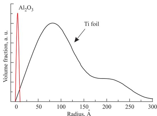
Fig. 9. Size distribution of scatterers in ion implanted titanium and corundum
