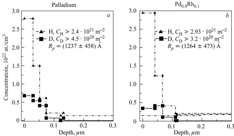
Fig. 7. The depth concentrations of D and H atoms after 25-keV  $D^+$  implantation at fluence  $\Phi_1 = 1.2 \cdot 10^{22} \text{ m}^{-2}$  in pure Pd (a) and  $Pd_{0.9}Rh_{0.1}$  (b) samples
