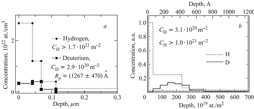
Fig. 12. The depth concentrations of D and H atoms after  $D^+$ -ion implantation with the energy of 25 keV at a fluence of  $\Phi_1 = 1.2 \cdot 10^{22} \text{ m}^{-2}$  in  $Pd_{0.9}Ag_{0.1}$  samples 10 days after (a) and three months later (b)
