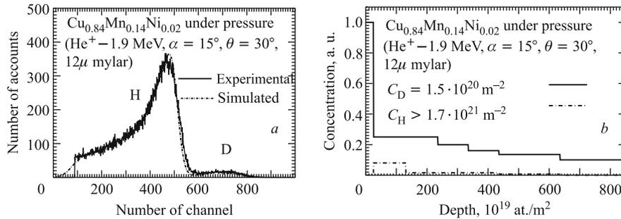
Fig. 3. The experimental and simulated spectra of H and D recoils measured by ERDA (*a*) and calculated depth concentrations of D and H atoms after saturation of manganese alloy sample under 9 kbar deuterium gas high pressure during 72 h (*b*). Measurements were carried out a long period of time after saturation
