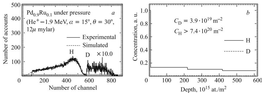
Fig. 2. The experimental and simulated spectra of H and D recoils measured by ERDA (*a*) and calculated depth concentrations of D and H atoms after saturation of  $\text{Pd}_{0.9}\text{Ru}_{0.1}$  alloy under 9 kbar deuterium gas high pressure during 72 h (*b*). Measurements were carried out a long period of time after saturation
