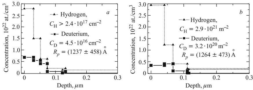
Fig. 11. The depth concentrations of D and H atoms after implantation of  $D^+$  ions with the energy of 25 keV at a fluence of  $\Phi_1 = 1.2 \cdot 10^{22} \text{ m}^{-2}$  in pure Pd (a) and  $Pd_{0.9}Ag_{0.1}$  (b) samples
