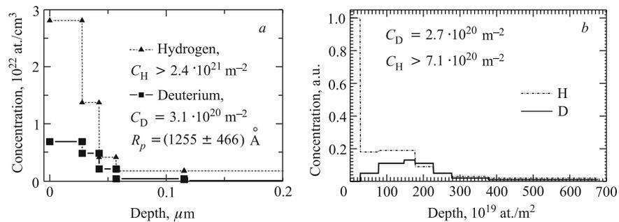
Fig. 15. The depth concentrations of D and H atoms after  $D^+$ -ion implantation with the energy of 25 keV at a fluence of  $\Phi_1 = 1.2 \cdot 10^{22} \text{ m}^{-2}$  in  $\text{Pd}_{0.9}\text{Ru}_{0.1}$  samples 10 days after (a) and three month later (b)
