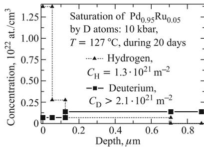
Fig. 7. ERDA depth concentrations of D and H atoms after saturation of annealed (at 125 °C, one hour)  $\text{Pd}_{0.95}\text{Ru}_{0.05}$  sample under 10 kbar deuterium gas high pressure during twenty days at temperature 127 °C. Measurements were carried out 5 days after saturation
