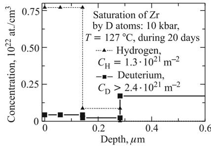
Fig. 8. ERDA depth concentrations of D and H atoms after saturation of annealed (at 125 °C, one hour) pure zirconium sample under 10 kbar deuterium gas high pressure during twenty days at temperature 127 °C. Measurements were carried out 5 days after saturation
