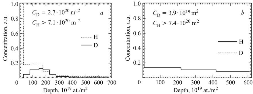
Fig. 9. ERDA depth concentrations of D and H atoms after implantation of D<sup>+</sup> ions up to a fluence of  $\Phi = 1.2 \cdot 10^{22} \text{ m}^{-2}$  (a) and saturation under 9 kbar deuterium gas during three days of Pd<sub>0.9</sub>Ru<sub>0.1</sub> sample (b). Measurements were carried out 30 days after saturation and implantation
