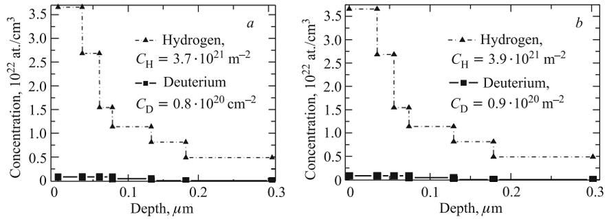
Fig. 4. ERDA depth concentrations of D and H atoms after saturation of annealed manganin sample (at 125 °C, one hour) under 9 kbar deuterium gas high pressure during 72 h. Measurements were carried out one month after saturation on the same sample just in different places ((a) and (b)) for detailed comparison of result repetition
