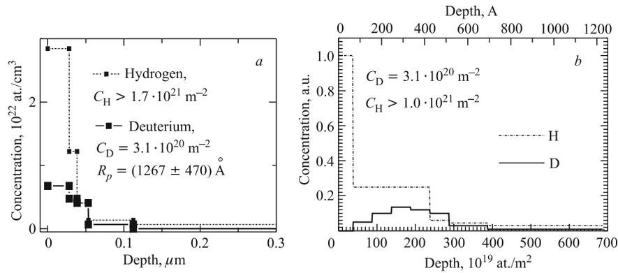
Fig. 13. The depth concentrations of D and H atoms after  $D^+$ -ion implantation with the energy of 25 keV at a fluence of  $\Phi_1 = 1.2 \cdot 10^{22} \text{ m}^{-2}$  in  $\text{Pd}_{0.9}\text{Pt}_{0.1}$  samples 10 days after (a) and three months later (b)
