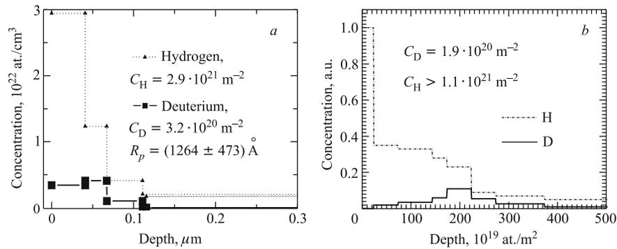
Fig. 14. The depth concentrations of D and H atoms after  $D^+$ -ion implantation with the energy of 25 keV at a fluence of  $\Phi_1 = 1.2 \cdot 10^{22} \text{ m}^{-2}$  in  $\text{Pd}_{0.9}\text{Rh}_{0.1}$  samples 10 days after (a) and three month later (b)
