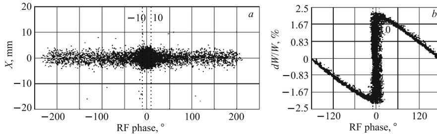
Fig. 8. Saw-tooth buncher impact on the beam at the inflector entrance (a) and midplane (b)
