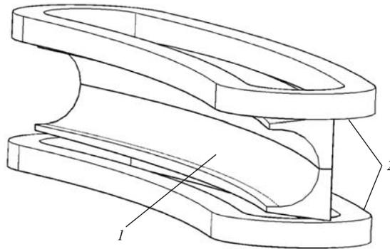
Fig. 15. Active gradient corrector: 1 — iron; 2 — coils
