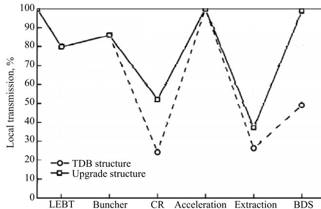
Fig. 17. Partial transmission (exit/entrance beam intensity ratio)
