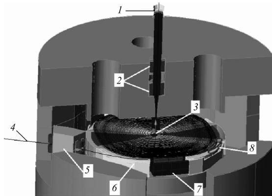
Fig. 1. Computer model of the HITFiL cyclotron: 1 — buncher; 2 — solenoids; 3 — inflector; 4 — reference particle trajectory; 5 — magnetic channel (M2); 6 — magnet sector; 7 — electrostatic deflector (ES1); 8 — harmonic coil
