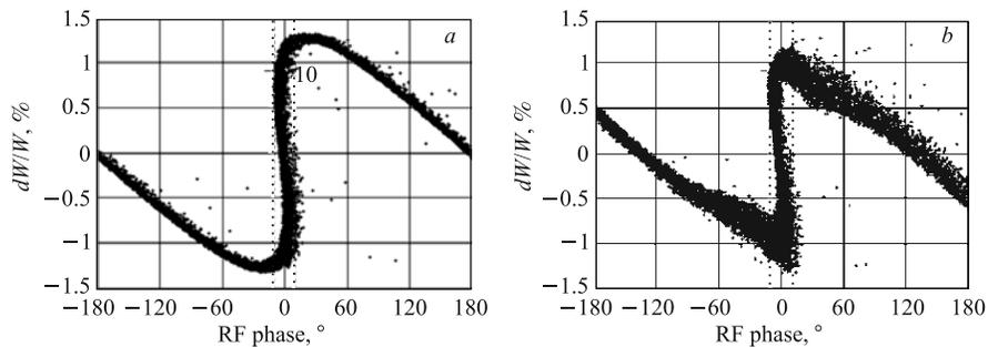
Fig. 6. Midplane longitudinal ion distributions with the incident beam intensity  $0 e \cdot \mu\text{A}$  (a) and  $200 e \cdot \mu\text{A}$  (b) for the sine-wave buncher
