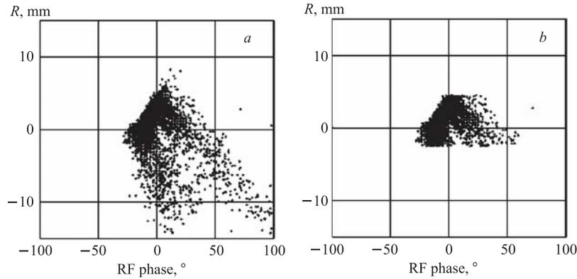
Fig. 11. Phase slit impact on the beam. There are beam projections in the place of the slit installation without the phase slit (a) and with the slit (b);  $R$  is the deviation of the ion radius from the reference value
