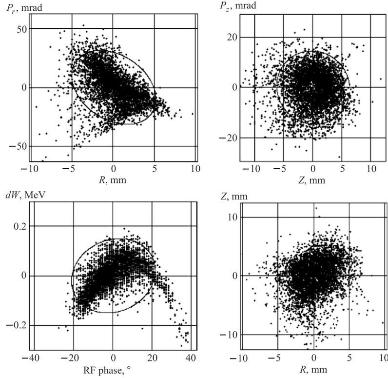
Fig. 12. Beam projections after completion of the 3rd turn ( $\theta = 270^\circ$ ) for the case with the phase slit:  $P_r$  is the radial momentum divided by the total particle momentum;  $R$  is the radius;  $P_z$  is the axial momentum divided by the total particle momentum;  $Z$  is the  $Z$ -coordinate;  $dW$  is the deviation of the ion energy from the reference value. The solid line ellipses have half-axes equal to 2 standard deviations of the corresponding distributions
