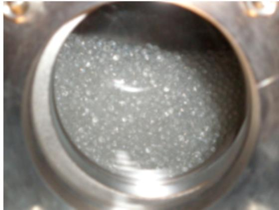
Fig. 3. Photo of the cold solid beads of mesitylene at  $T \sim 40$  K inside the chamber-imitator of the moderator chamber
