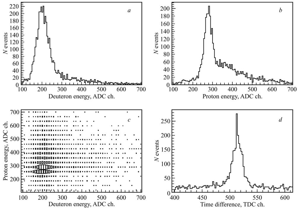
Fig. 3. Data obtained with polyethylene target at 880 MeV: distributions of the amplitudes for scattered deuterons (*a*) and recoil protons (*b*). The correlation of the amplitudes (*c*) and time difference between signals for proton and deuteron detectors (*d*)
