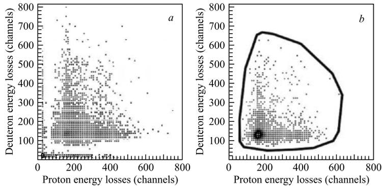
Fig. 5. Correlations of proton and deuteron energy losses: *a*) without TDC gates, *b*) with TDC gates. ADC criterion is presented by the solid line
