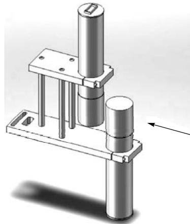
Fig. 2. Detector for registration of protons and deuterons
