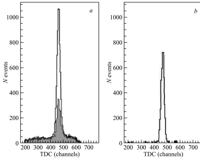
Fig. 7. Procedure of  $\text{CH}_2$ -C subtraction (*a*) and result of subtraction (*b*). White spectra are  $\text{CH}_2$  data, gray spectra are C data
