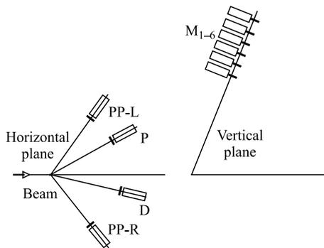
Fig. 1. Scheme of the experimental setup at the internal target station: P — proton detector; D — deuteron detector; PP-L and PP-R are the detectors for  $pp$ -quasi-elastic scattering;  $M_{1-6}$  — monitor counters
