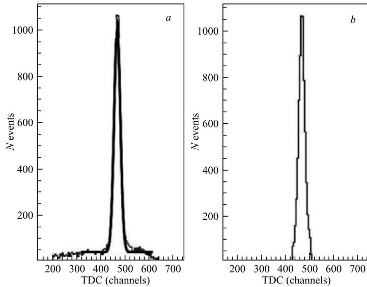
Fig. 4. Application of the gates on deuteron–proton time difference spectra: *a*) spectra without gates, *b*) spectra with gates. The fit is presented by the solid line
