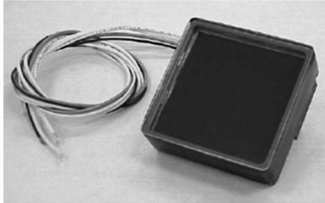
Fig. 2. View of MCP-PMT XP85012
