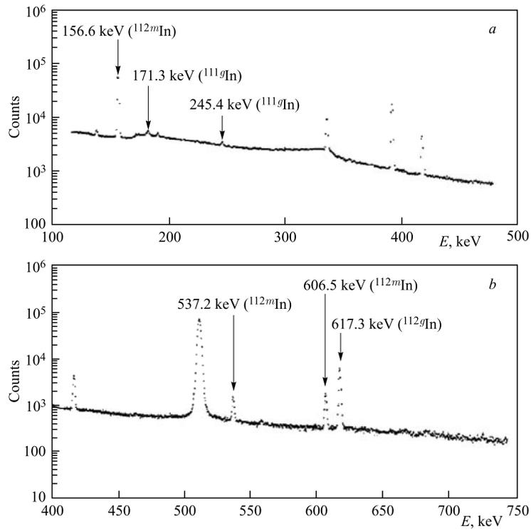
Fig. 2. A typical gamma spectrum of natural indium irradiated by 24 MeV end-point energy bremsstrahlung
