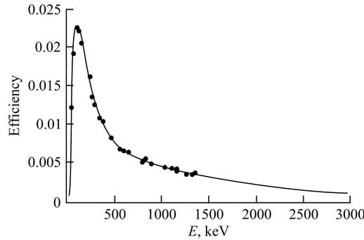
Fig. 1. The efficiency of the HP(Ge) semiconductor detector measured at a distance of 5 cm
