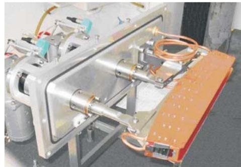
Fig. 14. Passive magnetic channel
