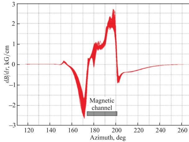
Fig. 17. Radial gradient of magnetic field on the trajectories of ions during extraction. Horizontally defocusing gradient of fringe field on the azimuths 155–175° is changed by focusing one in the aperture of the magnetic channel 175–200°
