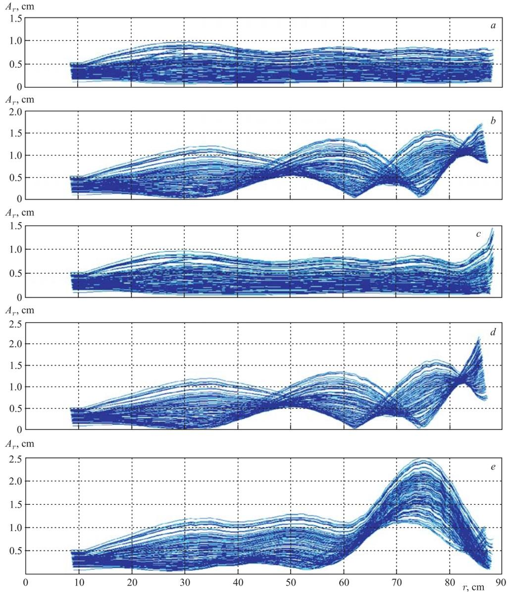
Fig. 11. Amplitudes of the radial oscillations for 200 ions depending on the average radius of orbits. *a)* No perturbations of magnetic field; *b)* 1st harmonic is in the field; *c)* 2nd harmonic is in the field; *d)* 1st and 2nd harmonics are in the field; *e)* 1st and 2nd harmonics are in the field and harmonic windings are also switched on
