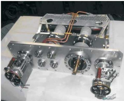
Fig. 13. Electrostatic deflector
