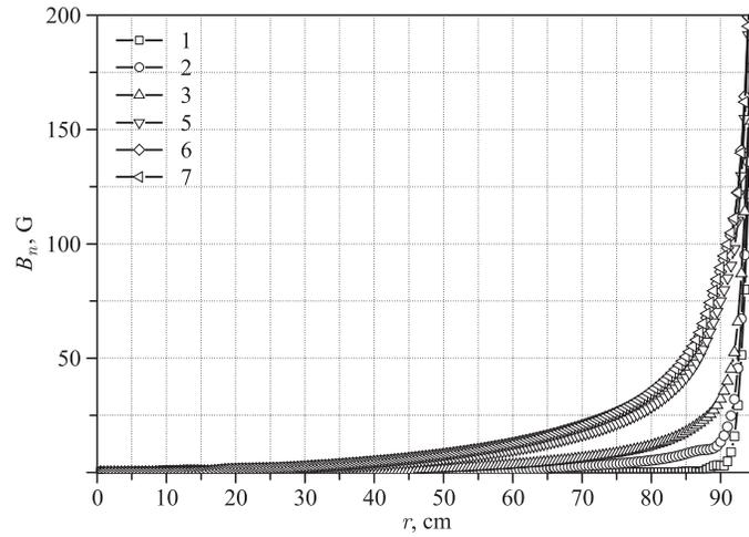
Fig. 4. Harmonic amplitudes of imperfections in calculated field without false channel. If false channel is installed, then the odd harmonics will disappear while the even ones will be doubled
