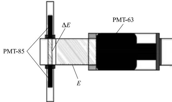
Fig. 1. Sketched view of  $\Delta E-E$  detector
