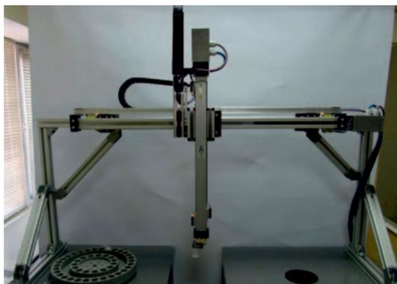
Fig. 2. General view of the sample changer
