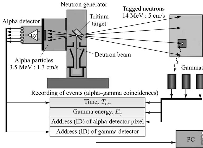
Fig. 1. Tagged neutrons device
