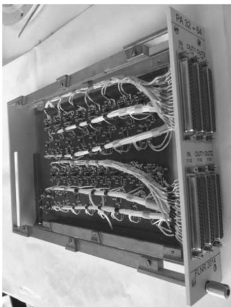
Fig. 1. PA32-64 — 32-input splitter-amplifier module
