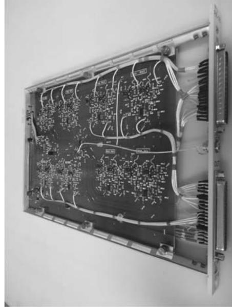
Fig. 2. 16-channel charge-sensitive preamplifier with autocalibration mode
