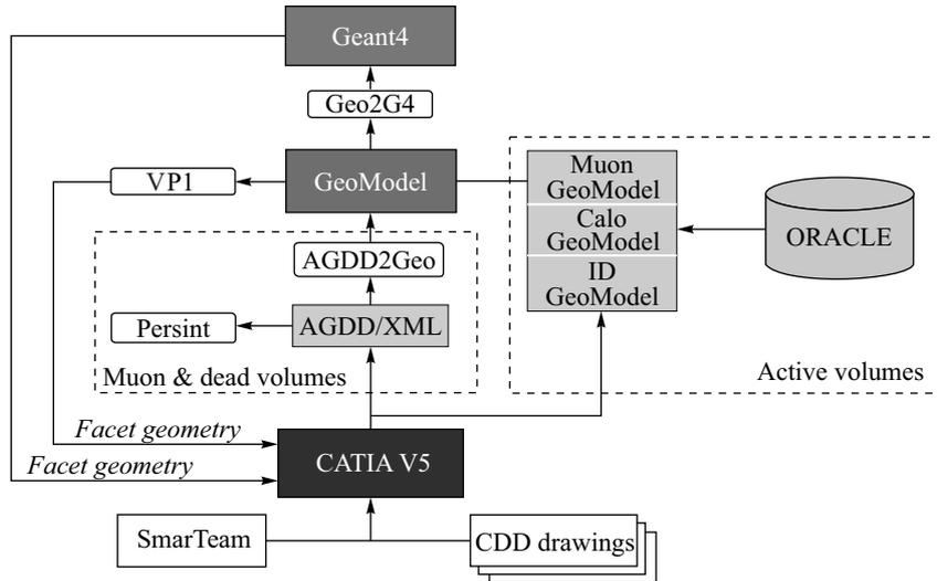
Fig. 2. ATLAS simulation loop with CATIA
