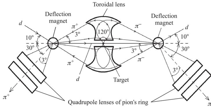
Fig. 1. Sketch of the pion production section with toroidal lens
