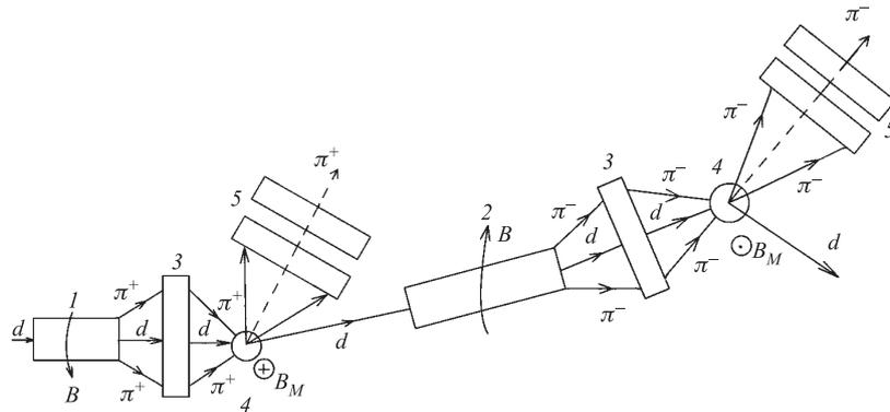
Fig. 3. Sketch of the pion production section with two magnetized targets. 1 is the first magnetized pion production target applied for positive pion collection; 2 is the second magnetized pion production target used for collection of the negative pions; 3 are the quadrupole lenses; 4 are the dipole deflection magnets; 5 are the quadrupole lenses of the pion ring
