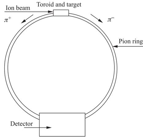
Fig. 2. Sketch of the pion–pion collision experiment
