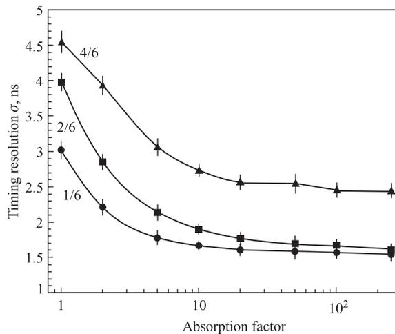
Fig. 6. CSC timing resolution for different majority coincidence options as a function of the absorption factor
