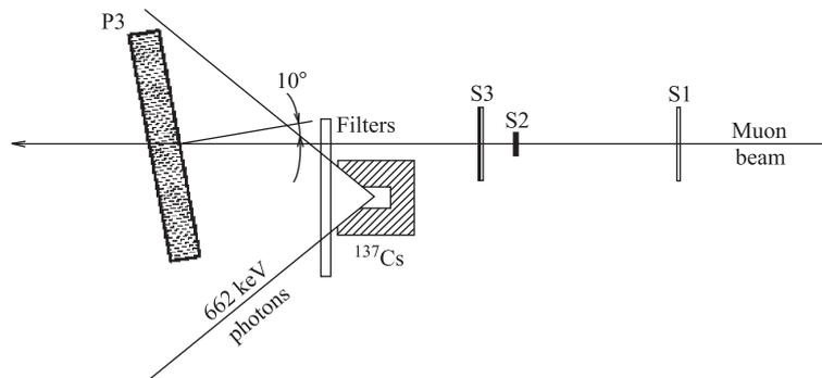
Fig. 2. Experiment layout (top view)
