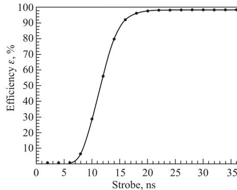
Fig. 5. CSC registration efficiency vs. strobe width for 4/6 majority scheme
