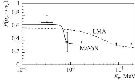
Fig. 3.  $P(\mu_e \rightarrow \nu_e)$  vs  $E_\nu$  for MaVaN [32] oscillations (solid curve). The dashed curve corresponds to conventional oscillations with the best-fit solution to KamLAND data
