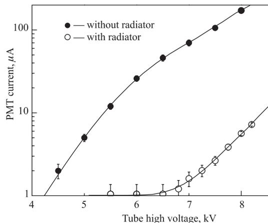
Fig. 4. Results of the test measurements with and without the TRD radiator
