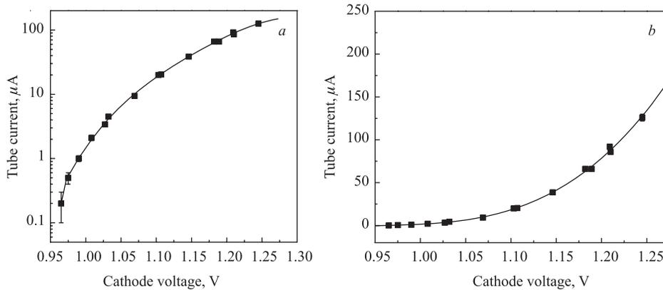
Fig. 2. Dependence of the tube current on the cathode voltage
