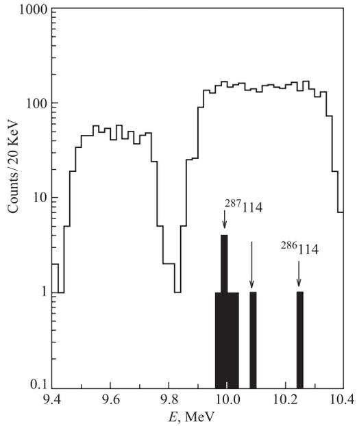
Fig. 2. Spectrum of  $Z = 114$  ( $A = 287$ ) detected alpha decays
