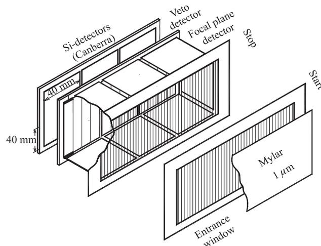
Fig. 1. The detection module of the DGFRS
