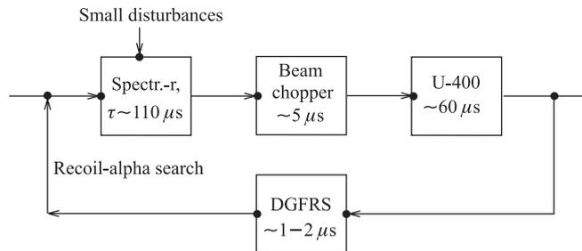
Fig. 3. Flow chart of the whole real-time process which is applied for radical suppression of background products in SHE element synthesis experiments [7]
