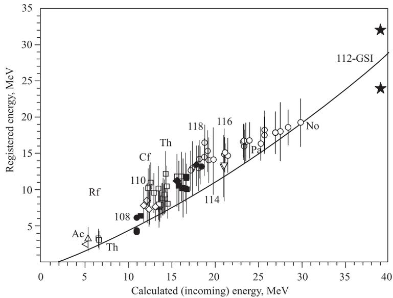
Fig. 4. The dependence of registered heavy-recoil energies against calculated incoming ones for the DGFRS detecting module. The line corresponds to calculations [8] for  $^{288}114$  recoil. Two events of  $Z = 112$  element synthesized at GSI [9] are shown by stars. Note, that efficiency of Rf recoil detection by silicon detector was not close to  $\sim 1$
