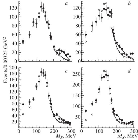
Fig. 3. The missing mass of the  $p(e, e'p)X$  reaction [16] studied at JLAB in Hall C at  $Q^2 = 4.0 \text{ GeV}^2$ . The open circles correspond to Monte-Carlo simulations; the full circles correspond to data. *a*–*d* correspond respectively to  $p_p^0 = 2 \text{ GeV}$  and  $\theta_p^0 = 23^\circ$ ,  $p_p^0 = 2 \text{ GeV}$  and  $\theta_p^0 = 20^\circ$ ,  $p_p^0 = 2.2 \text{ GeV}$  and  $\theta_p^0 = 17^\circ$ , and  $p_p^0 = 2.45 \text{ GeV}$  and  $\theta_p^0 = 17^\circ$
