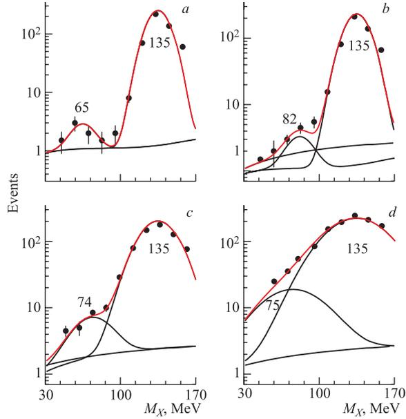
Fig. 6. Missing mass spectra for  $pp \rightarrow ppX$  measured at SATURNE (SPES3 beam line) at  $T_p = 1520$  MeV.  $a-d$  correspond respectively to the following spectrometer angles:  $\theta_{\text{spec}} = 0, 2, 5,$  and  $9^\circ$
