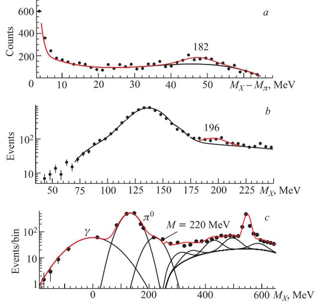
Fig. 2. *a*)  $\pi^0$  electroproduction at threshold, measured at MAMI [13]. The missing mass spectra are integrated over 4 channels. *b*) Missing mass of the  $p(e, e'p)\pi^0$  reaction studied at JLAB in Hall A at  $\theta_{\text{cm}} = 90^\circ$  [14]. *c*) Missing mass of the  $p(e, e'p)X$  reaction measured at JLAB in Hall C [15]
