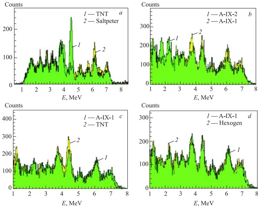
Fig. 10. The energy spectra of  $\gamma$  quanta for different explosives: a) TNT (1) and saltpeter (2); b) A-IX-2 (1) and A-IX-1 (2); c) TNT (1) and A-IX-1 (2); d) A-IX-1 (1) and hexogen (2)
