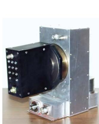
Fig. 3. The box of the frontend electronics of the alpha detector mounted on a neutron generator with ground target
