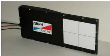
Fig. 5. The profilometer to measure spatial distributions of the neutron tagged beams. The working area is marked by the white sheet with the cross
