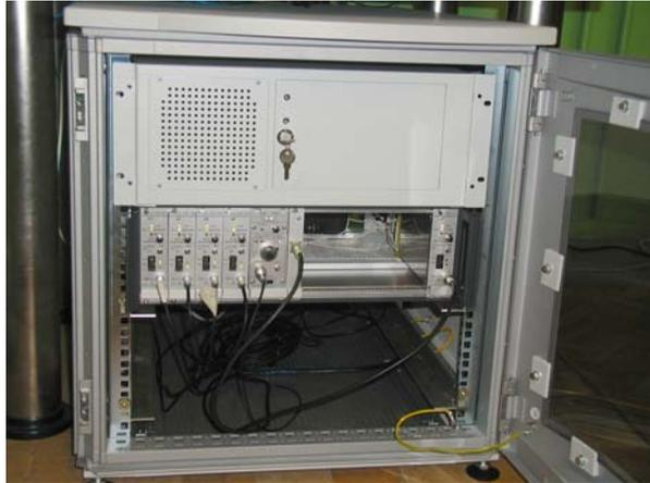
Fig. 8. The DAQ system and the detector power supply
