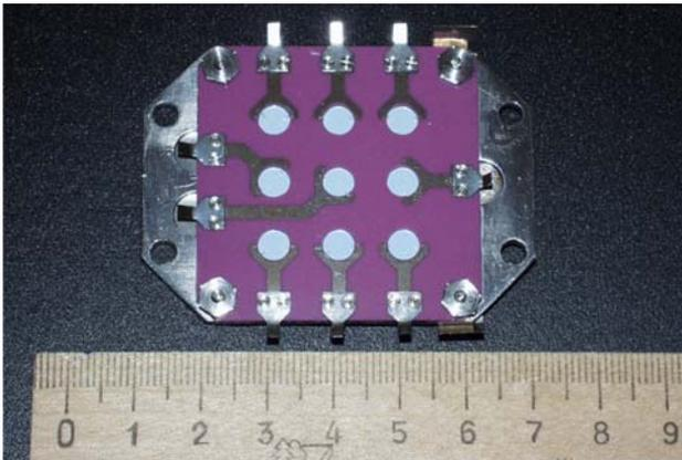
Fig. 2. Nine-pixel alpha detector viewed from the back
