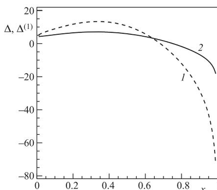
The deviation of the electron spectrum in muon decay from the spectrum in the Born approximation: for the lowest order  $\Delta^{(1)}$  (1), for all orders  $\Delta$  (2) of perturbation theory
