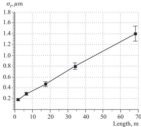
Fig. 9. Dependence  $\sigma_t(L)$  on the distance covered by laser beam in the plugged tube; a telescopic collimating attachment and a rotating prism are used
