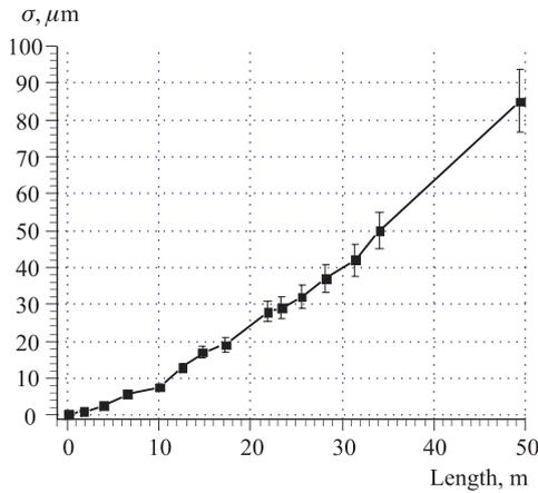
Fig. 6. Uncertainty  $\sigma(L)$  in the spatial position of the laser beam axis as a function of the distance covered by the beam in the air; no collimator was used
