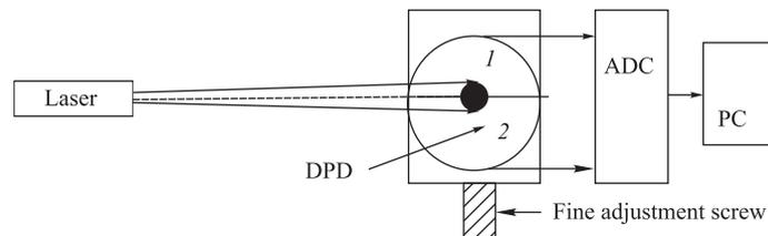
Fig. 1. Block diagram of the setup for measuring the uncertainty  $\sigma(L)$  in the spatial localization of the laser beam
