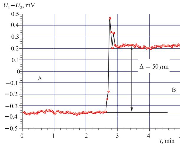
Fig. 4. Record of the laser beam «position» on the dee photodetector after the travel over a distance of 34 m in a tube plugged with optical glasses; calibration shift  $\Delta = 50 \mu\text{m}$
