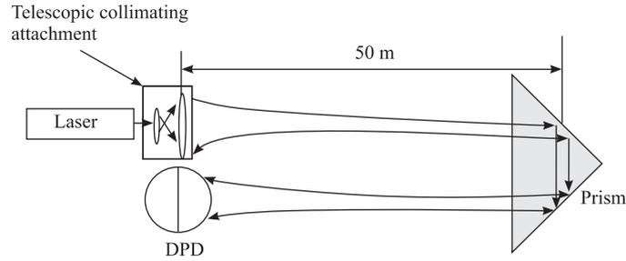
Fig. 3. Collimation of the laser beam in the experiment with lengths over 50 m
