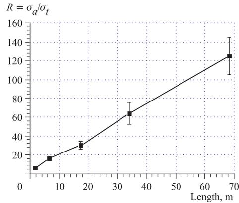
Fig. 10. Dependence of the «resolution improvement» coefficient  $R(L)$  on the laser beam travel length
