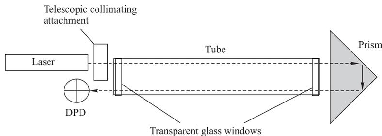
Fig. 8. Experimental layout with the plugged tube
