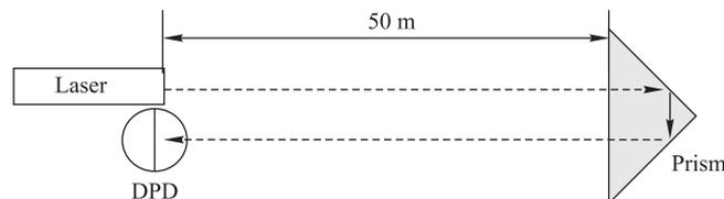
Fig. 2. Experimental layout for lengths over 50 m in the air
