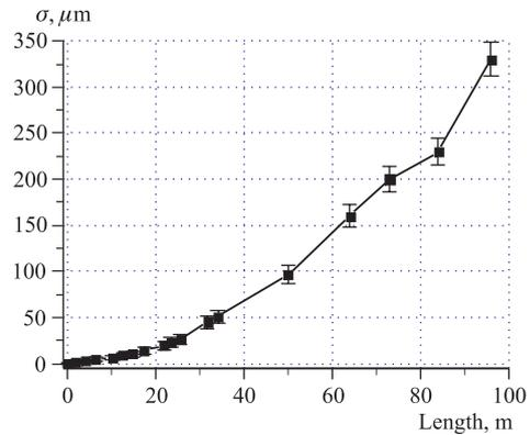
Fig. 7. Uncertainty  $\sigma(L)$  in the spatial position of the laser beam axis as a function of the distance covered by the beam in the air; a telescopic collimating attachment and a rotating prism are used
